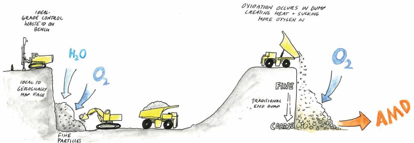
Figure 7 – the drill, blast, load and haul of PAF can cause AMD, particularly with large end dumps.
