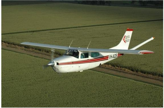
A Cessna Series 210L, VH-JHF were used as the survey platforms. These aircraft combine good maneuverability with the benefits of a magnetically clean base for minimal interference with the magnetic performance of the sensor.
