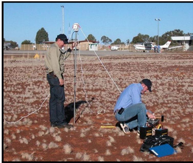
Figure 11 Setting up base station magnetometer
