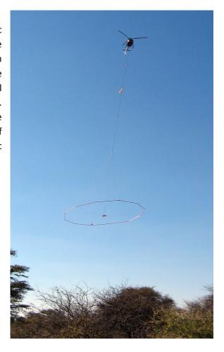
The system was designed to be field configurable to best suit a large variety of different geophysical requirements from deep penetration to optimizing the discrimination within a narrow range of resistivity values.
