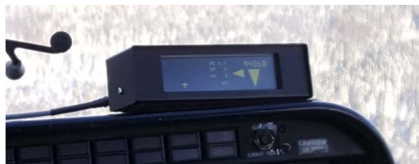
Figure 3. Pilot Steering Indicator and Radio Altimeter Indicator
