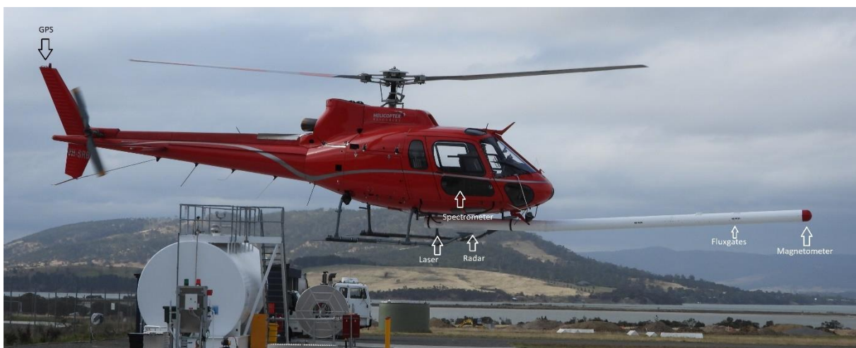
Figure 2.1: Photo of the survey aircraft showing the location of the sensors (e.g. alkali vapour magnetometer; Schedule 3: 1.9a), fluxgate magnetometer (Schedule 3: 1.9a), gamma-ray spectrometer, radar altimeter, laser altimeter, GNSS antennas).
