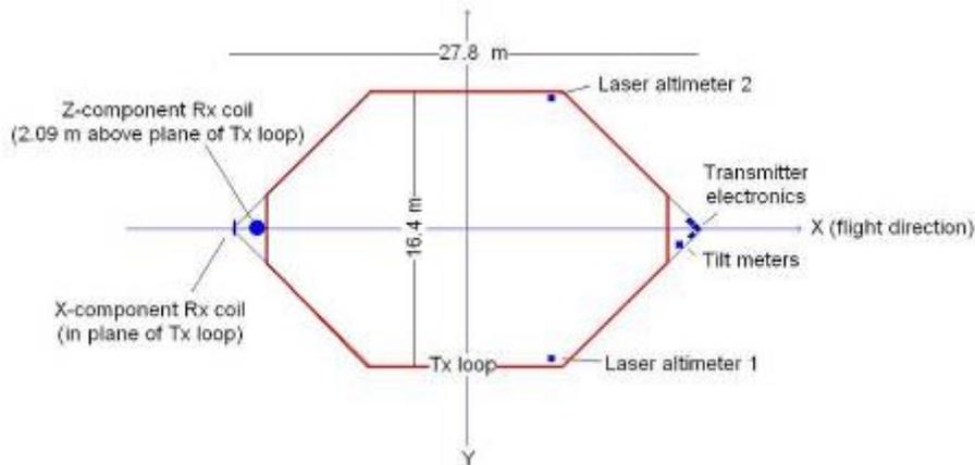
Figure 2 Sketch showing the Tx frame and instrument locations for a configuration with Tx loop area of 314 m<sup>2</sup>.
