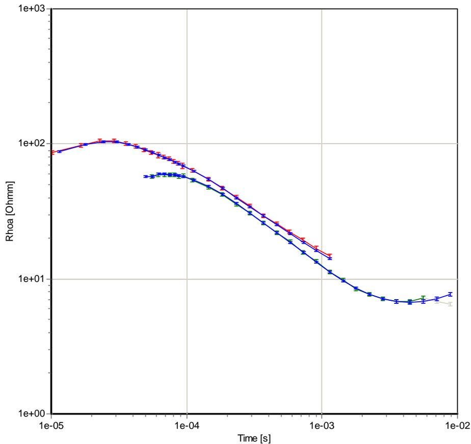
Figure 6. Calibration Data from 15 m altitude at the National Danish Reference site, presented as apparent resistivity vs delay time. The blue curves are the response related to the ground based systems and the green and the red curves are the measured data with the SkyTEM system. The error bars are 2%.
