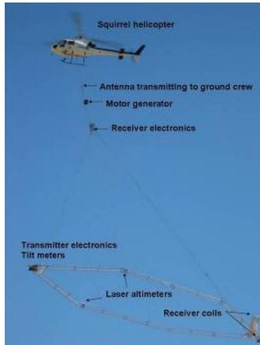
Figure 1 Photo of SkyTEM in operation at Toolibin Lake, Western Australia, October 2006. Transmitter area is 314 m<sup>2</sup>.
