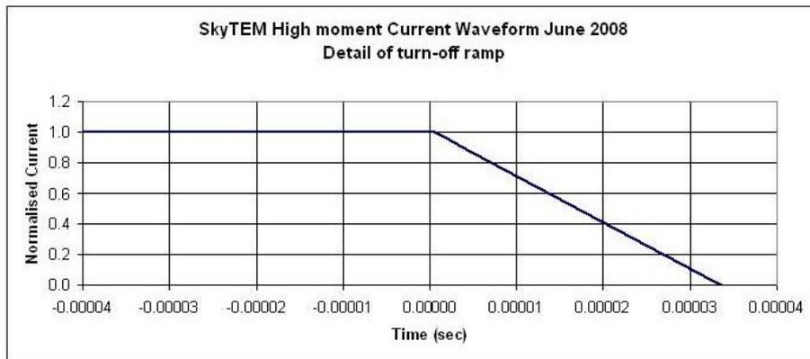
Figure 3 Piecewise linear approximation to the high moment transmitter waveform, plotted as a fraction of peak current (typically 100A). Panel a) shows the on-time of the HM current waveform. b) shows detail of the current turn-off ramp. The total turn-off ramp is typically 38  $\mu$ s, depending on peak transmitter current.
