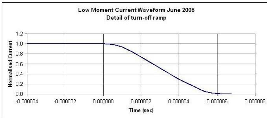
Figure 4 Piecewise linear approximation to the low moment transmitter waveform, plotted as a fraction of peak current (typically 40A). Panel a) shows the on-time of the LM current waveform. b) shows detail of the current turn-off ramp. The total turn-off ramp is approximately 6  $\mu$ s.
