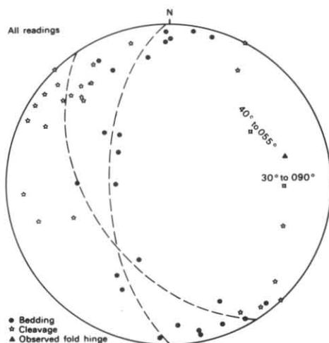
Figure 8. Stereographic plot of structural data, Haunted Bay area.
