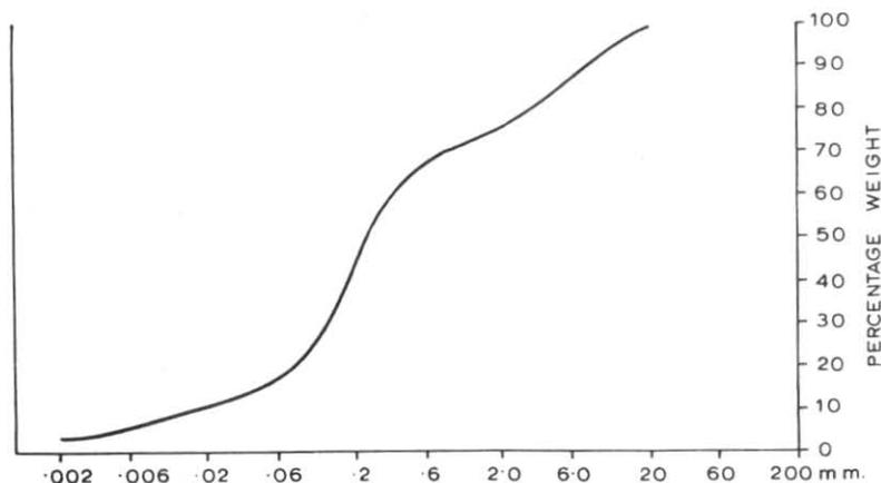
FIGURE 6.—Cumulative curve of washed layer in moraine from wall of canal at pumping station on SE shore of Lake St Clair.
