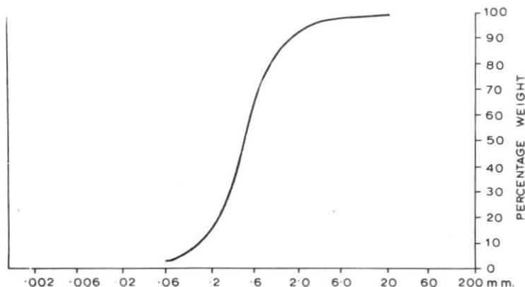
FIGURE 4.—(Top) Section in crest of retreatal end moraine, 400 yards SE of Cynthia Bay, Lake St Clair. (Bottom) Cumulative curve of gravelly sand at point "A" in section.
