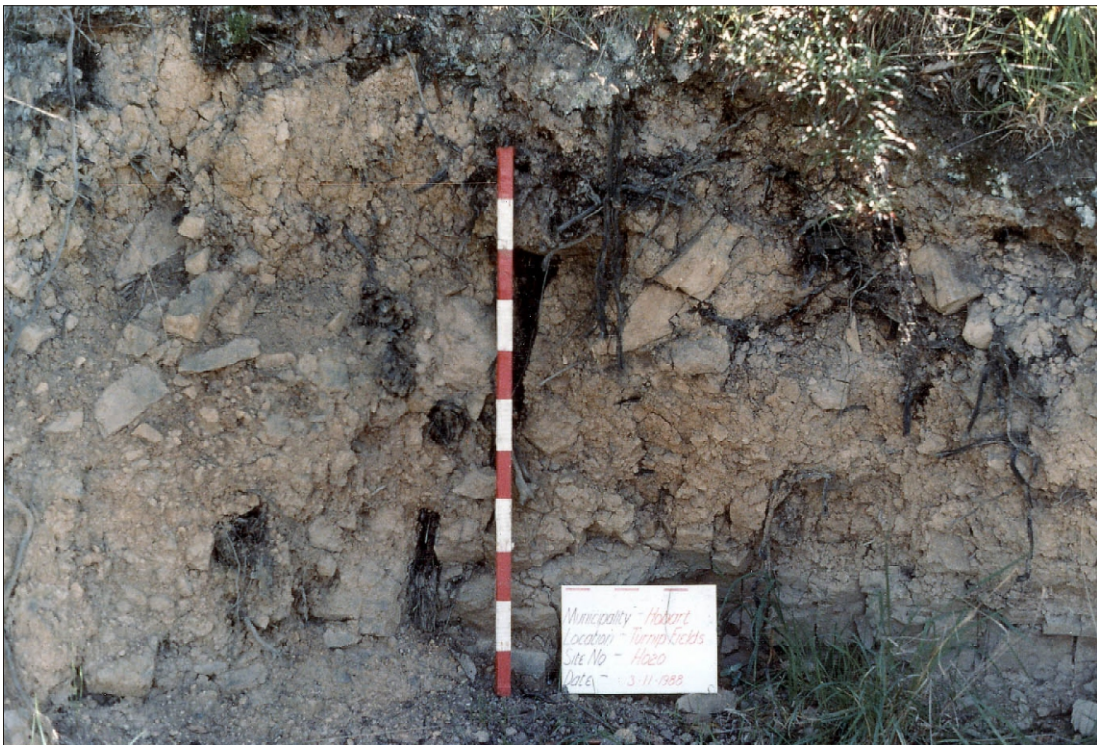
Plate 2. Sandy gravel slope deposits on Permian bedrock — Turnip Fields, Fern Tree
