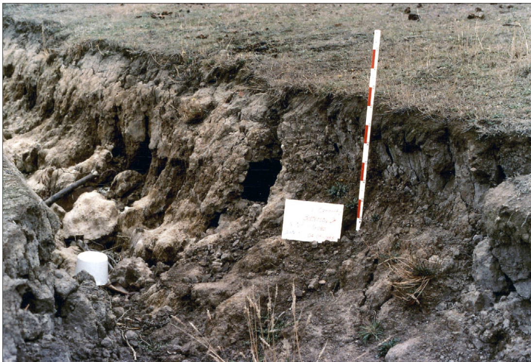
Plate 5. Tunnel erosion in soils on Triassic sediments — Battersby Drive, Glenorchy
