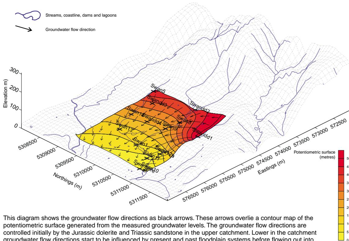
This diagram shows the groundwater flow directions as black arrows. These arrows overlie a contour map of the potentiometric surface generated from the measured groundwater levels. The groundwater flow directions are controlled initially by the Jurassic dolerite and Triassic sandstone in the upper catchment. Lower in the catchment groundwater flow directions start to be influenced by present and past floodplain systems before flowing out into Little Swanport.
