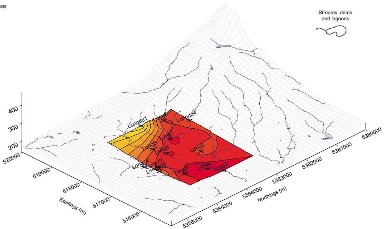
These two figures illustrate the shallow depth at which the groundwater sits below the ground surface. The piezometers indicate that the average depth to the water table is 3.09 metres. The lower diagram shows the effect of a high rainfall event on the catchment when the water table rose to an average depth of 2.80 metres.
