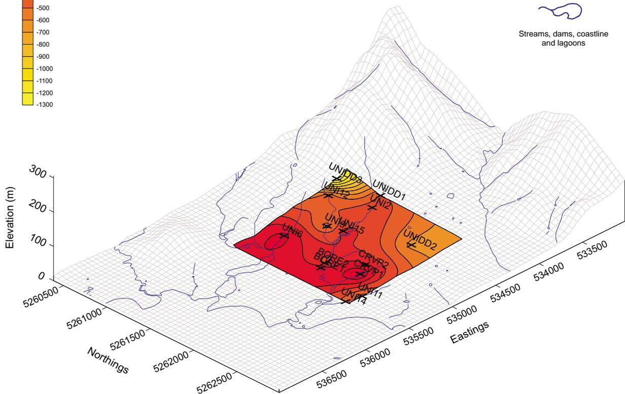
These two figures illustrate the depth at which the groundwater sits below the ground surface. The diagrams show deeper depths to groundwater higher in the catchment system around piezometers Uni12 and Uni9 and piezometers UniDD1, 2 and 3. Groundwater comes close to the ground surface close to the main drainage lines within the catchment, particularly around piezometers CRVP1, Bore1 and 2, and Uni6.
