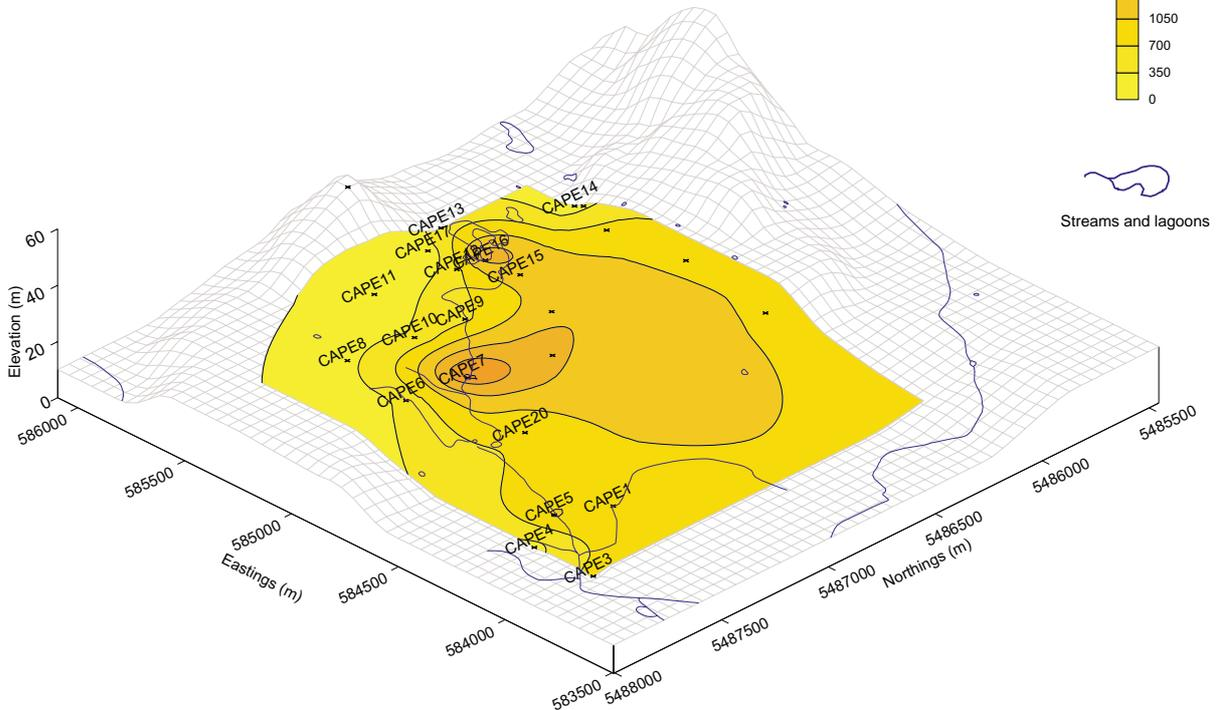
The important features to note on these diagrams are the extensive areas of moderately to severely saline soils centred around piezometer Cape 7 and to a lesser extent Cape 16. This surface area of salinisation correlates directly with the high levels of groundwater salinity observed in Figure 8. The surface soil salinity levels are lower than the average soil profile values which can be attributed to leaching of salts from the upper, more porous sandy soil profile.
