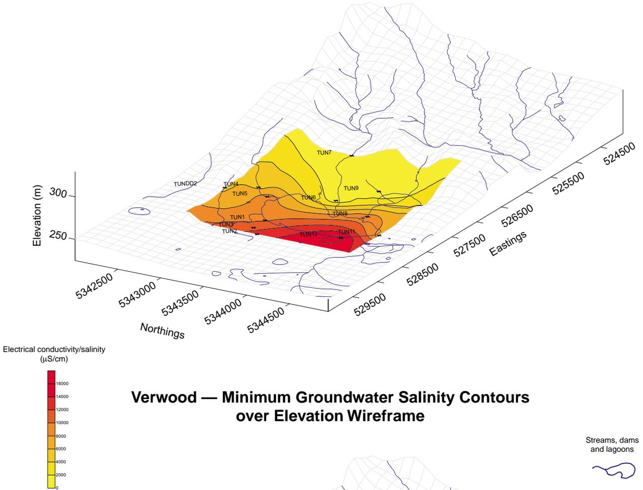
The important features to note on these diagrams are the areas of moderate to severe saline groundwater (4000–16 000  $\mu\text{S}/\text{cm}$ ) centred around Bar Lagoon at piezometers 1, 2, 3 and 12. Low salinity ground and surface water flow into the lagoon system from the west as measured by piezometers 6, 7 and 9. The lower diagram shows less severe saline groundwater, particularly within piezometers adjacent to Bar Lagoon, after a large rainfall event during November 1998.
