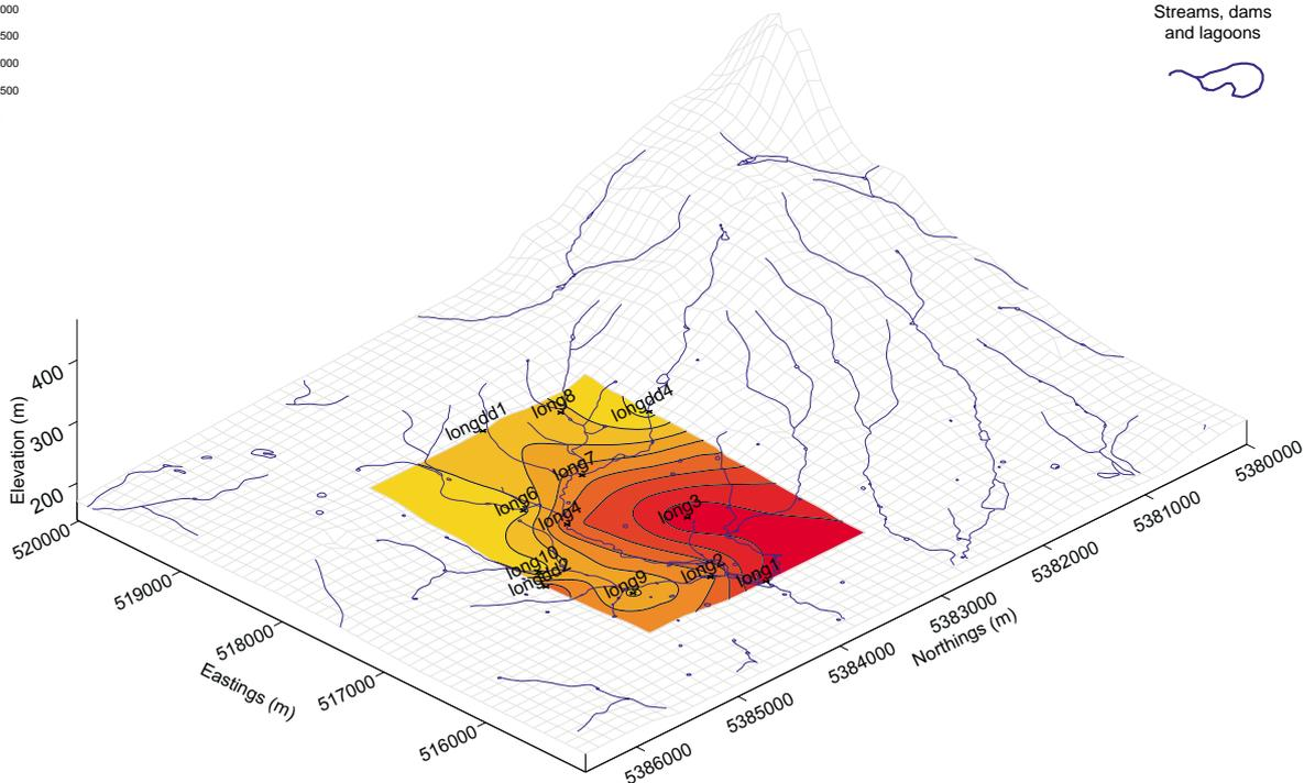
These diagrams show high average groundwater salinity levels about holes Long1 and Long3. This area corresponds to an area of subdued topography, and in the case of Long1 a large salt scald. The lower diagram shows the effect of a high rainfall event with a considerable influx of fresh groundwater into the northern and eastern part of the catchment.
