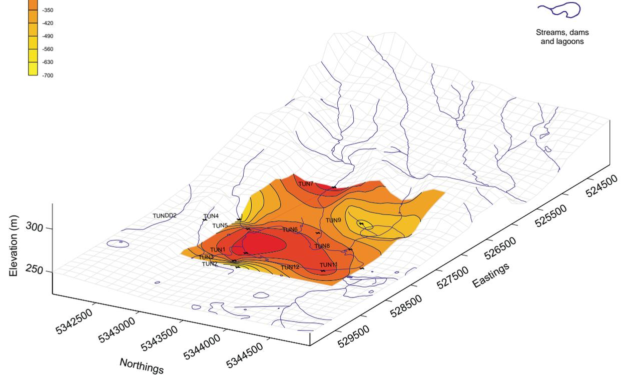
These two figures illustrate the shallow depth at which the groundwater sits below the ground surface. The piezometers indicate that the average depth to the water table is 3.4 metres. The lower diagram shows the effect of a high rainfall event on the catchment (109 mm) during November 1998 when the watertable rose to an average depth of about 3 metres. The most obvious feature is the large area of shallow groundwater and surface water around Bar Lagoon.
