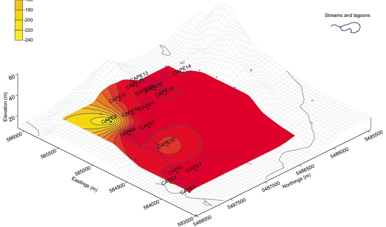
These two figures illustrate the shallow depth at which the groundwater sits below the ground surface. The piezometers indicate that the average depth to the water table is 1.1 metres. The lower diagram shows the effect of a high rainfall event on the catchment during January 2000 when the catchment water table rose to an average depth of just below 500 mm from the ground surface.
