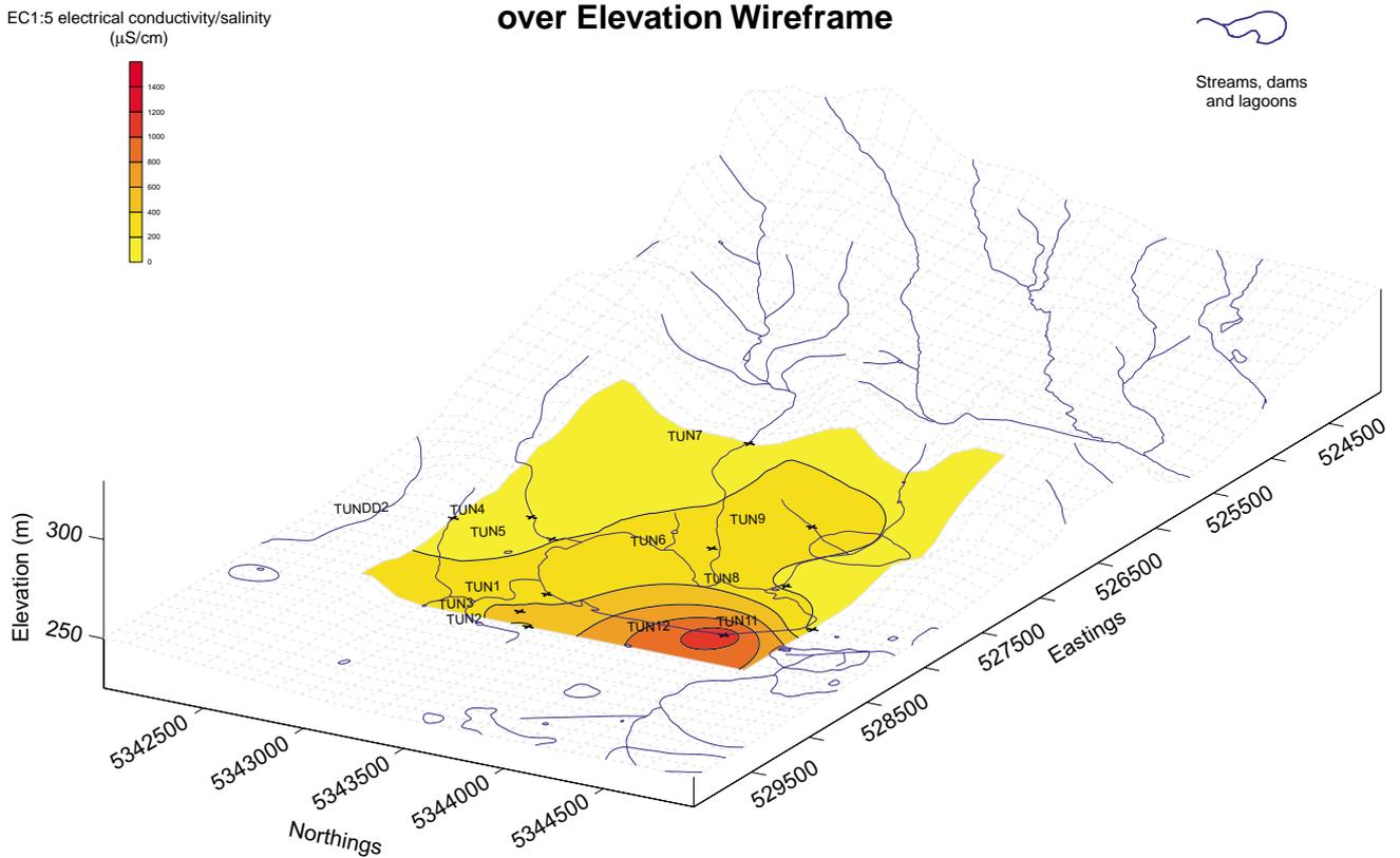
These diagrams clearly illustrate the high soil salinity levels present around Bar Lagoon, with the highest value centred around piezometer Tun12. Surface soil salinity levels are generally higher than average soil profile salinities, particularly close to Bar Lagoon. This is likely to be due to either near-surface evaporation concentrating salt within the upper two metres, or wind deposited salt contributing to observed high surface soil salinity levels.
