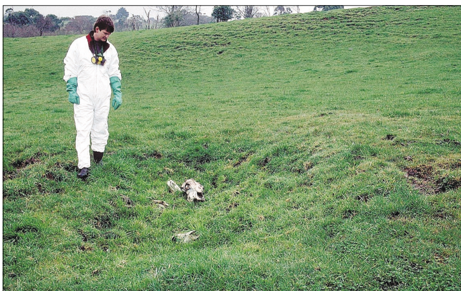
Plate 3. Subsidence related to the recent DAF trenches observed in the western part of the site.
