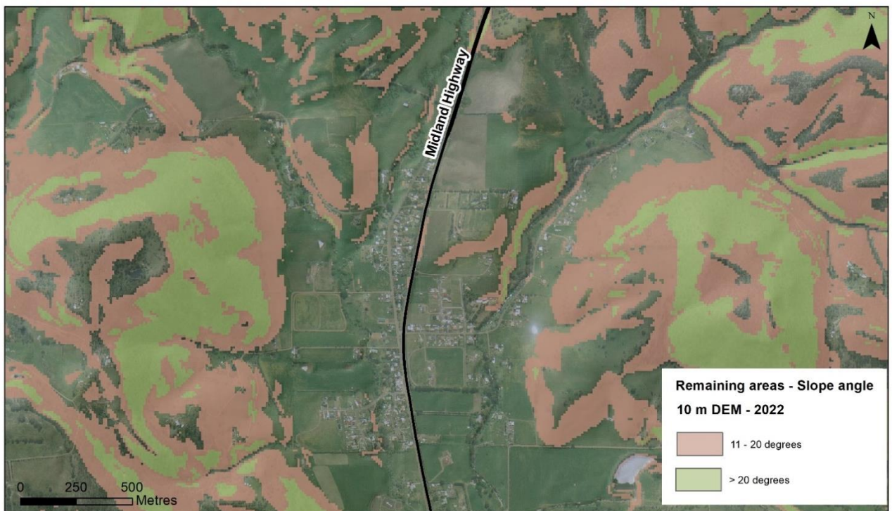
Figure 13. Slope angle categories (2013 methodology) mapped on the updated 10 m DEM.
