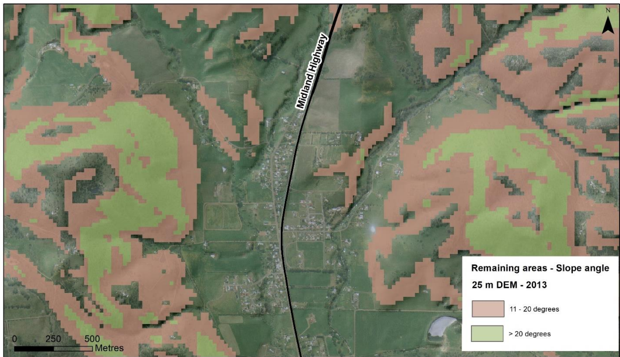
Figure 12. Remaining areas, slope angle components as mapped in 2013 using a 25 m DEM.
