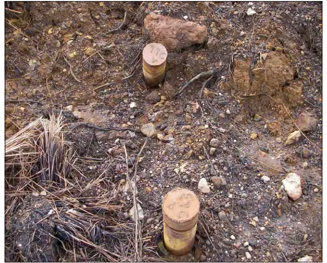
Steel collars — secure, sealed and permanent welded number.
