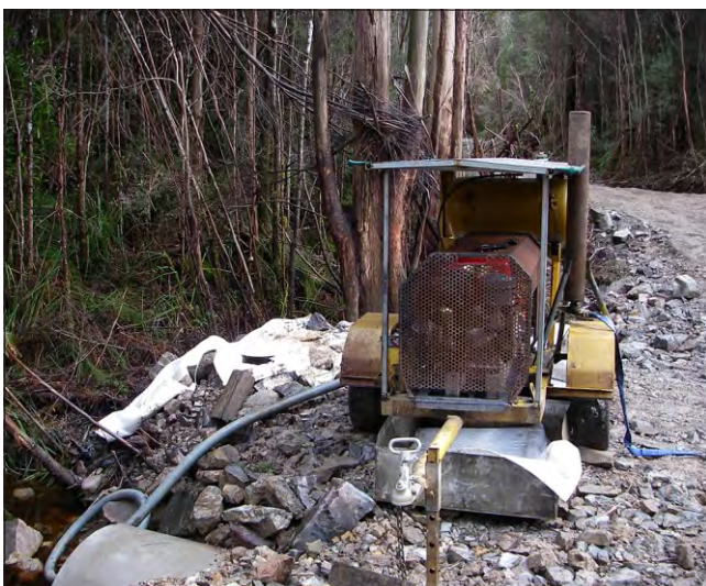
Roofed pump, fuel tank and bund.
