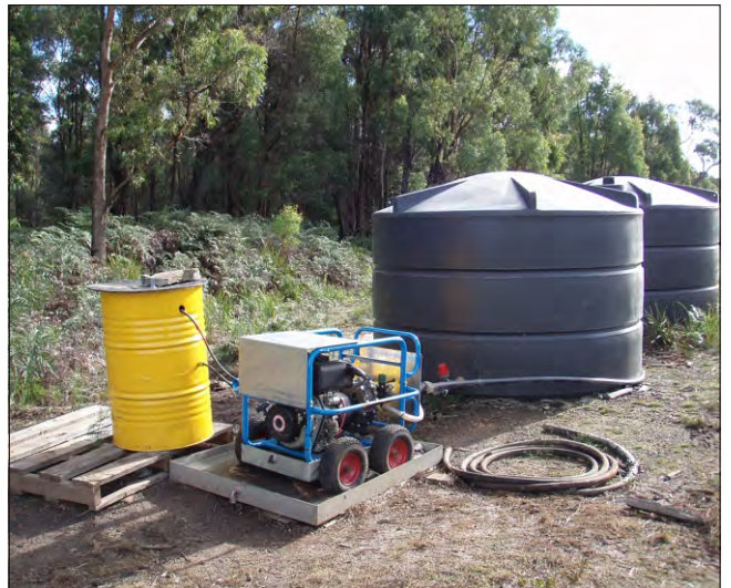
Excellent fuel tank setup contained within the yellow drum which acts as the bund.
