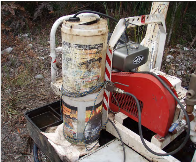
Poor bunding (filling with water) and jury rigged fuel supply to pump.
