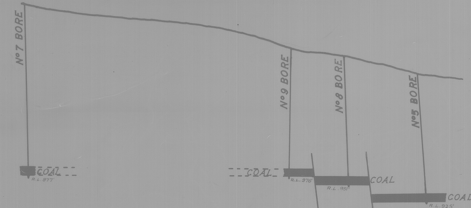
S-W SECTION THROUGH BORES 5, 8, 9, 7 SECTION 6
