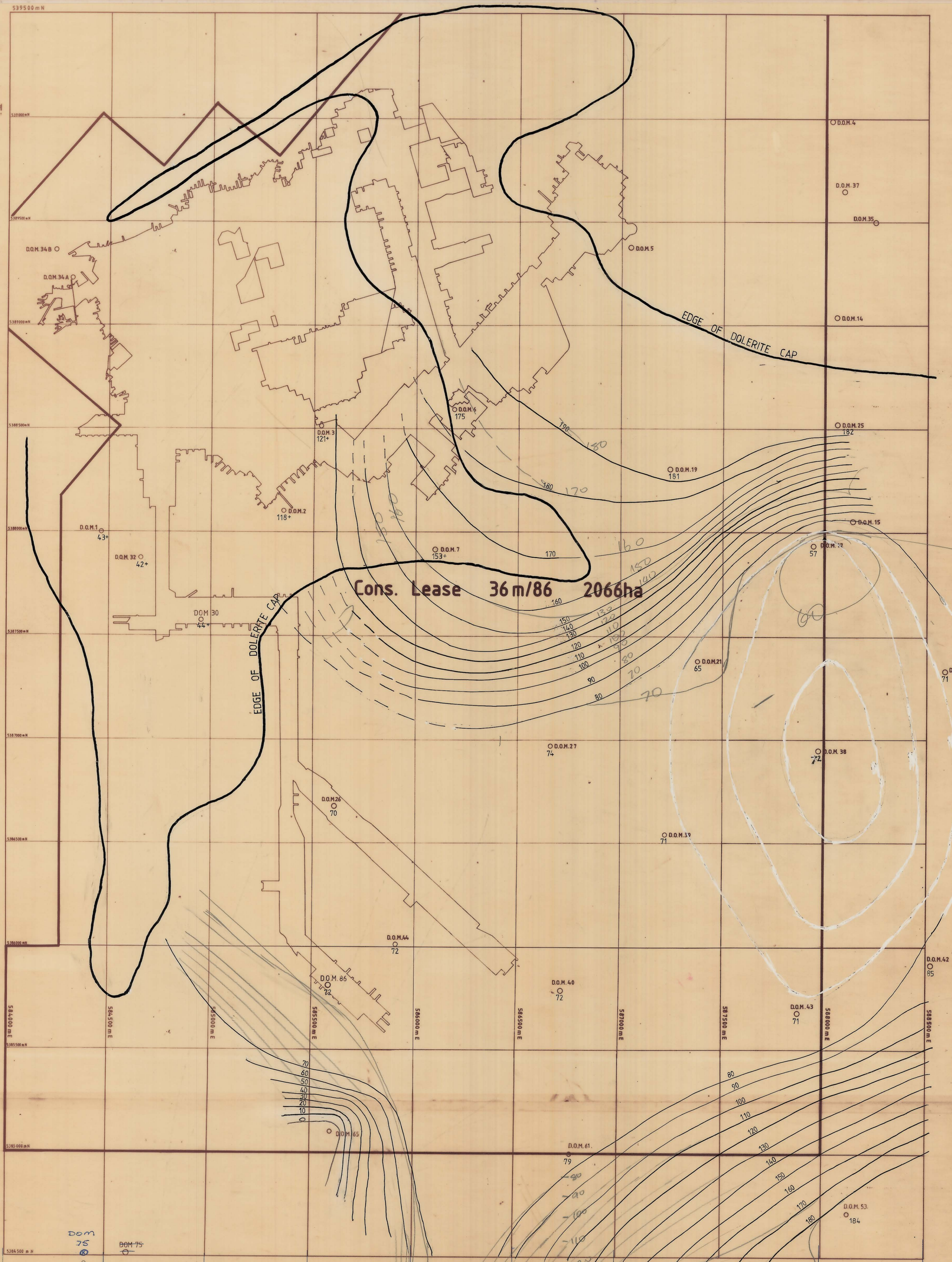
Thickness of sediments over Duncan seam and under dolerite cap. (Thickness in metres; where no cap present thickness of sediments under talus shown: 44+)
