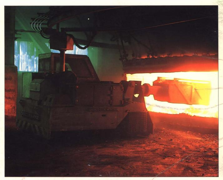
Electric trolley-wire charging car levelling the surface of the furnace charge with a silica/woodchip/coal mixture, Pioneer Silicon Industries, Electrona.
