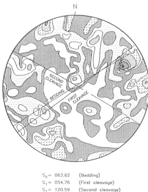
Figure 55. Quartz c-axes, 77/403. Re-oriented slide: 240.00. 153 measurements. Contours: 0.3, 1, 1.6, 2.3, 3, 3.6, 4.3% per 1% area.
