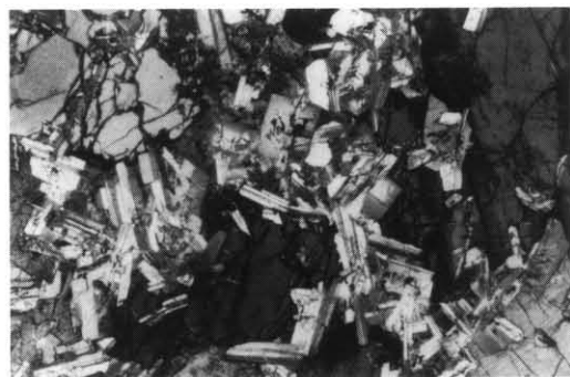
Plate 35. Thin section of sample from borehole 68, depth 58.7 m, Fingal Tier. Coarse-grained, moderately differentiated dolerite, showing ophitic to subophitic intergrowth of clinopyroxenes and plagioclase, grading into a finer feldspar-rich mesostasis. Crossed nicols, field of view 4.3 \times 2.9 mm.
