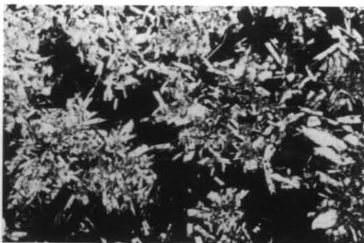
Plate 38. Thin section of sample 78/533 from EP858830. Fine-grained dolerite, plane-polarised light, \times 6.8 . Aggregates of intergranular plagioclase and clinopyroxene surrounded by dark, glassy, mesostasis.
