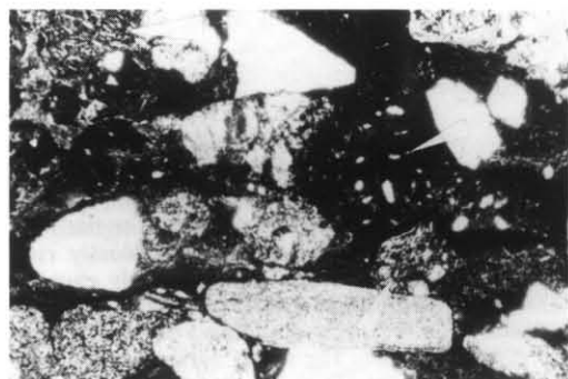
Plate 15. Coarse-grained lithic arenite. Thin section, \times 16 , plane-polarised light. Several trachytic-hyalopilitic volcanic rock fragments indicated by arrows. Sample E85, from FP032920.
