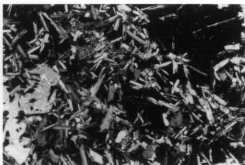
Plate C1. Sample M366, Tertiary tholeiitic basalt, Barnes Road, Showing an embayed olivine phenocryst (centre left), plagioclase laths, olivine and augite granules and black glass. Texture grades from hyalophitic (upper left) to intersertal or almost intergranular in less glass-rich areas (left). Crossed nicols. Field of view 4.3 \times 2.9 mm.
