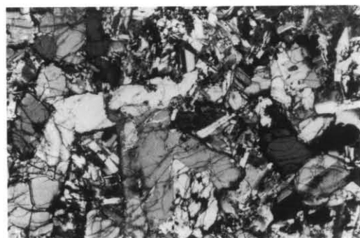
Plate 36. Thin section of sample from borehole 68, depth 214.8 m, Fingal Tier. Coarse-grained slightly differentiated dolerite, showing intergrown equant to columnar clinopyroxene crystal and finer feldspar-rich mesostasis. Texture intergranular to poorly-developed subophitic. Crossed nicols, field of view 4.3 \times 2.9 mm.
