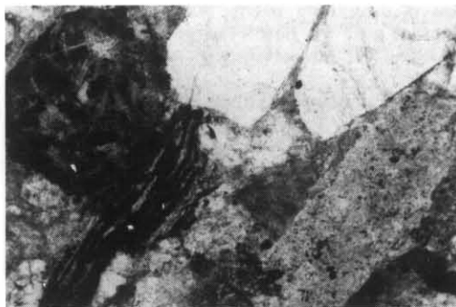
Plate 6. Photomicrograph (plane-polarised light) of sandstone in Ds. Width of the field of view is 1.55 mm. Clear grains of quartz with mottled grains of chert accompany a flake of carbonaceous shale and a grain of basic or intermediate volcanic material.
