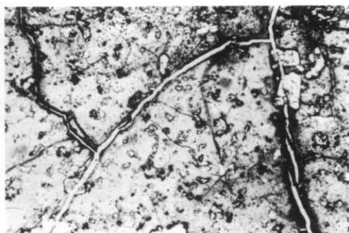
Plate 40. Thin section of glassy sedge of a late dolerite dyke. Sample TCE6, from EP899813. Larger phenocrysts of orthopyroxene, and smaller aggregates of clinopyroxene and plagioclase, in brown glass; zeolite veinlets. Plane-polarised light, x 6.8.
