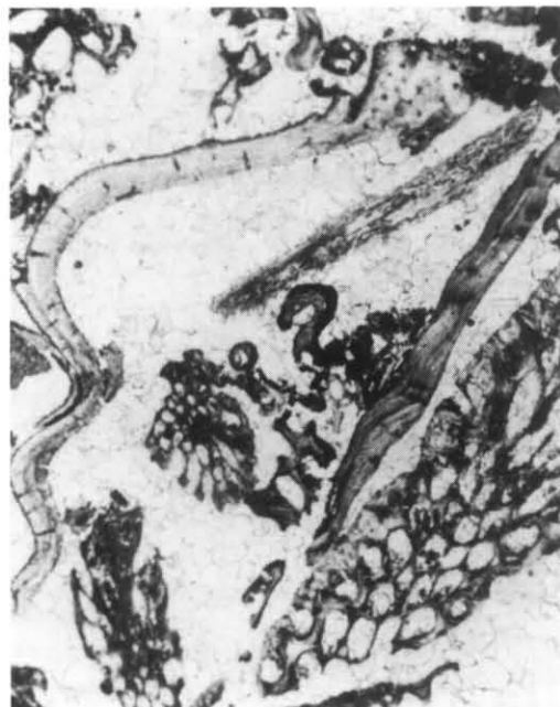
Plate 10. Thin section of coarse-grained calcarenite (x 12, plane-polarised light). Open, uncompacted fabric supported by coarse sparry calcite cement. Fossil fragments are predominantly bryozoans, with some punctate brachiopods and crinoids (lower left). Sample E324 [FP049908].
