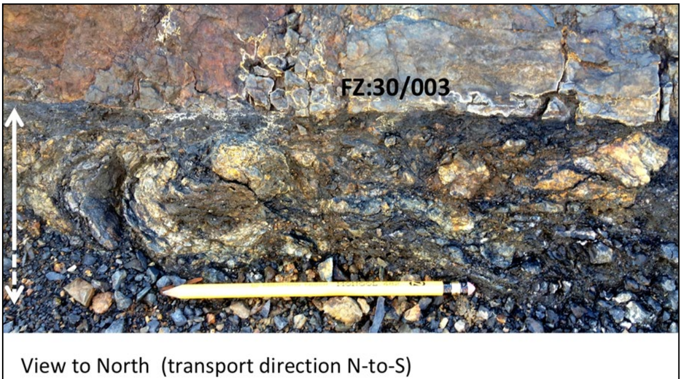
Figure 40. Mesoscopic fold in gouge breccia zone of décollement zone fault, Barren Knob Quarry. The fault has an attitude of 30^{\circ}/003^{\circ} (magnetic). Note partially continuous layering defining the fold hinge is truncated segmented with development of a fault breccia (right side of fault zone in photo).
