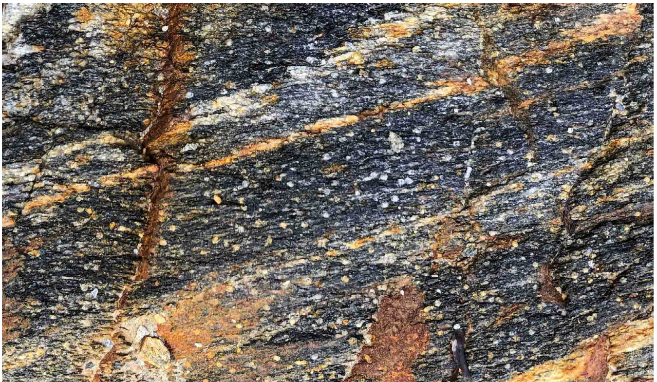
Figure 55. Laminated porphyroblastic albite-garnet schist typical of the high-grade Franklin metamorphic schists along the Mt McCall road (DG 19-62, Mt McCall road).
