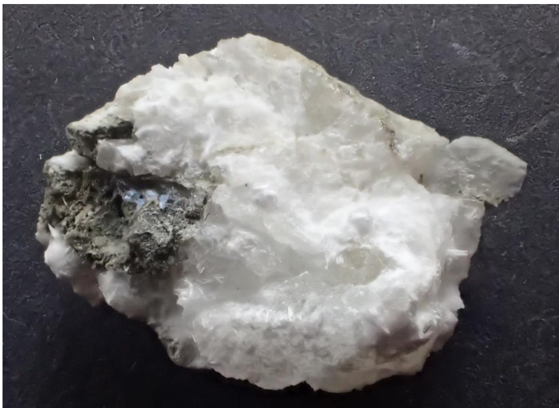
Figure 4: Sample G410118, Glassy white calcite plus white fibrous natrolite. Plain light, FOV (field of view) ~25mm.
