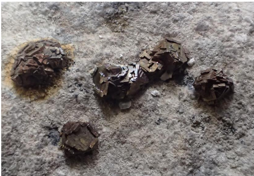
Figure 3: Sample G410112 Showing small spheroids of pyrite on matrix. Plain light, FOV (field of view) ~30mm.
