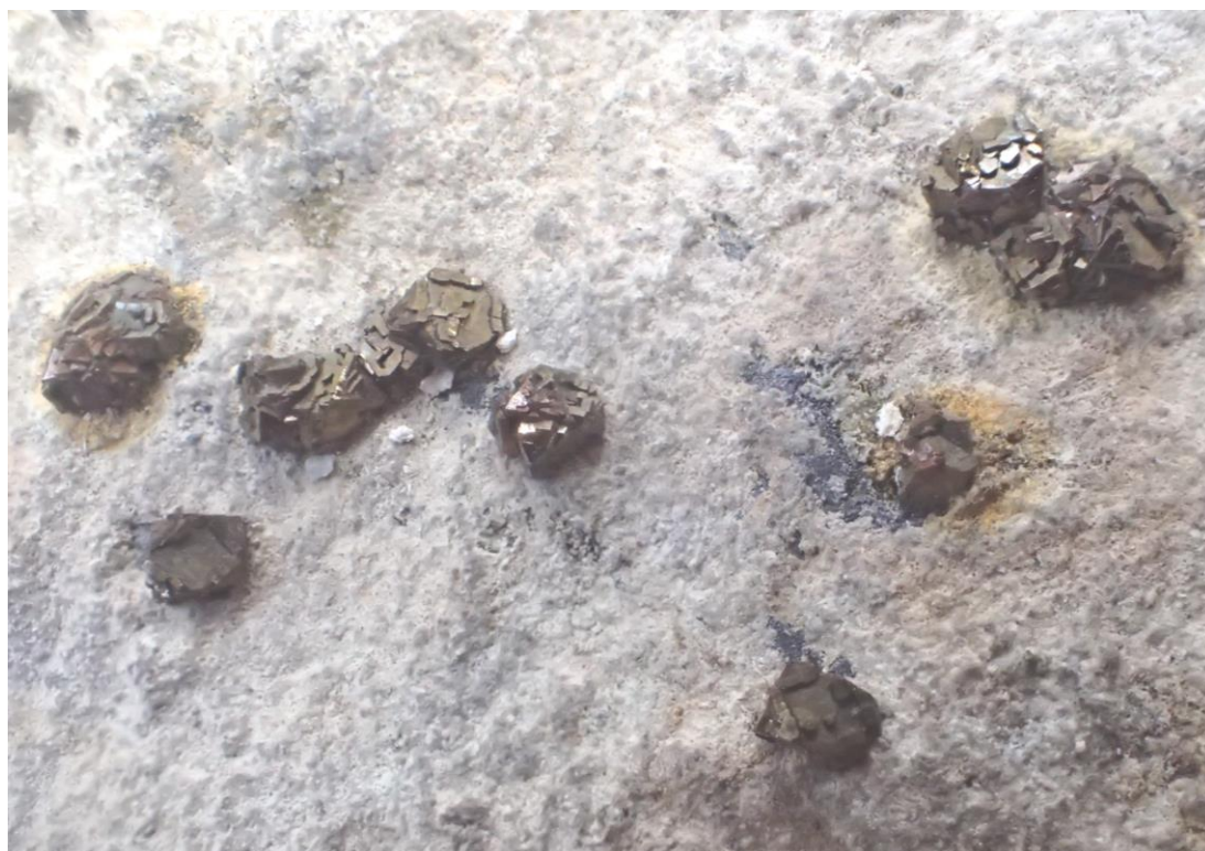
Figure 2 Sample G410112 Showing small spheroids of pyrite on matrix. Plain light, FOV (field of view) ~50mm.
