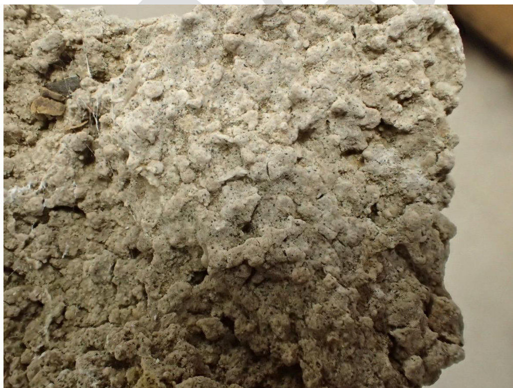
Figure 2: Sample as received, showing surficial cracking. Sample G410119. FOV: about 60 mm.
