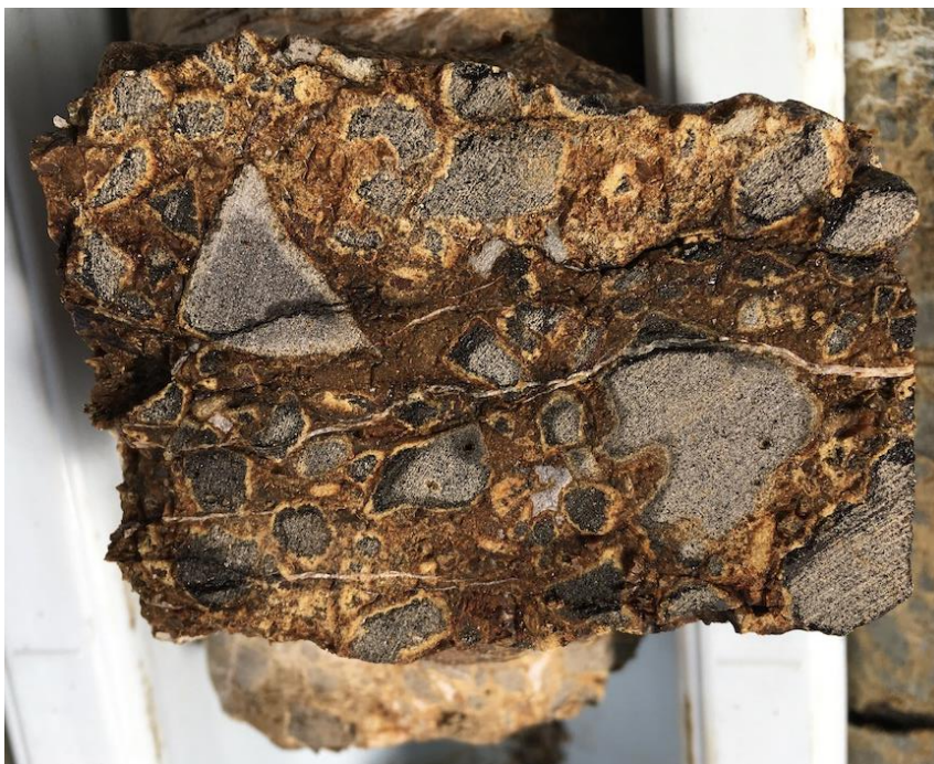
Fig. 4. G409322 BWBBH08/10.1 Basalt Breccia with brown hisingerite cement. FOV ~8cm.
