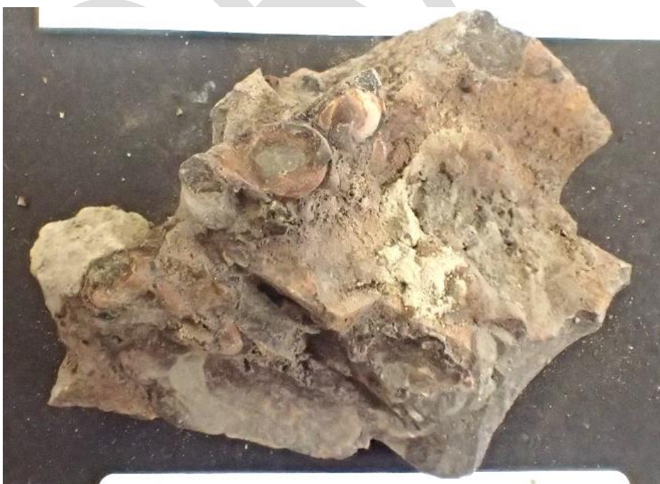
Fig. 7. G409324 BWBBH08/46.8 Basalt Breccia with carbonate coatings. FOV ~8cm.
