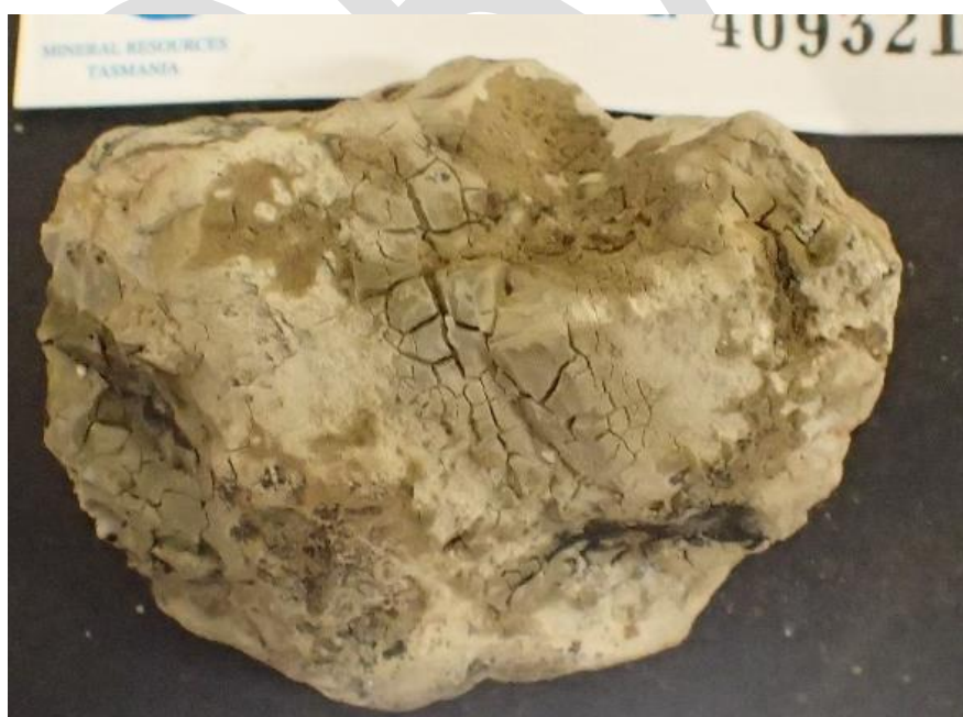
Fig. 3. G409321 BWBBH08/19.1 Clay patches in brecciated basalt. FOV ~ 85mm.
