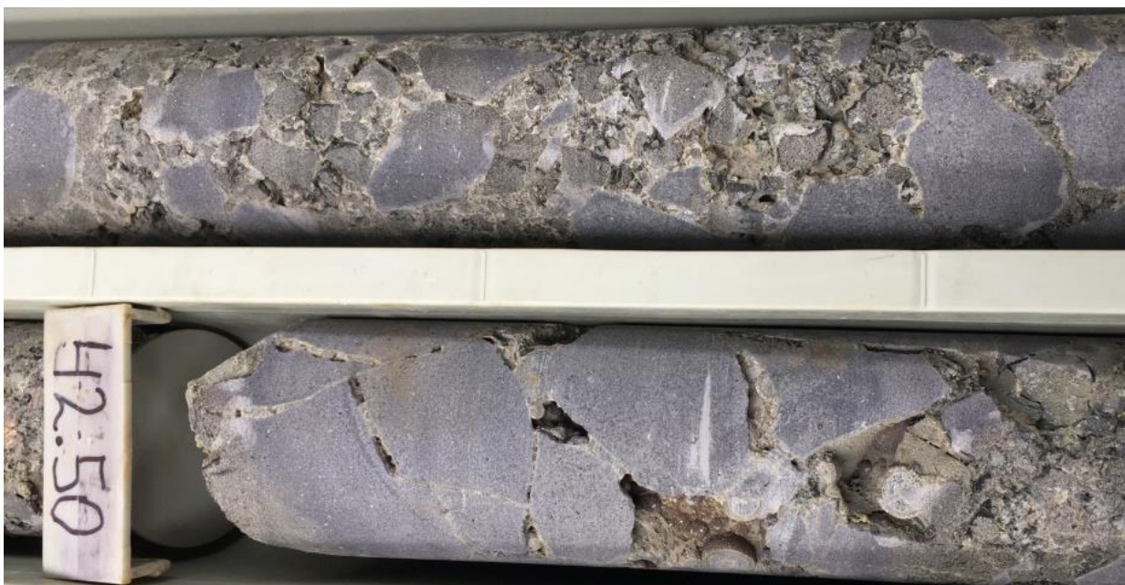
Fig. 6. G409324 BWBBH08/46.8 Basalt Breccia with cavities containing carbonates. FOV ~30cm.
