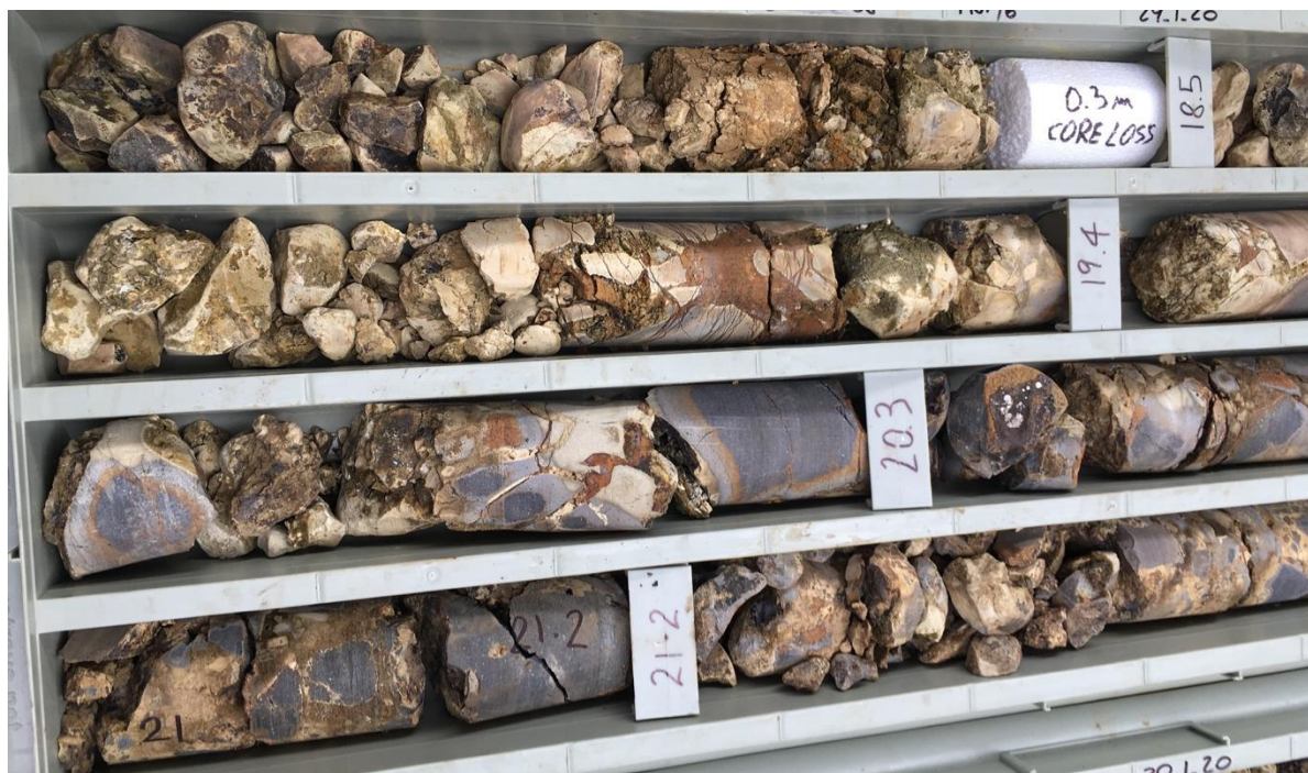
Fig. 2. G409321 BWBBH08/19.1 Clay patches in brecciated basalt. FOV ~ 1m.
