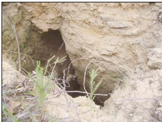
Figure 8. Typical small shaft with covering vegetation removed – 1200 mm x 900 mm and open to 8 metres.
