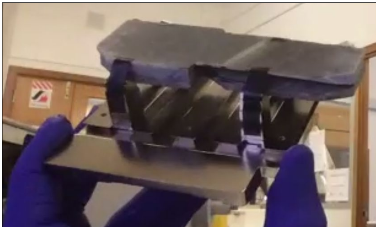
Figure A3.1. A polished and carbon-coated sample mounted in a holder that has been minutely adjusted, aligning the sample so it is level in the SEM.
