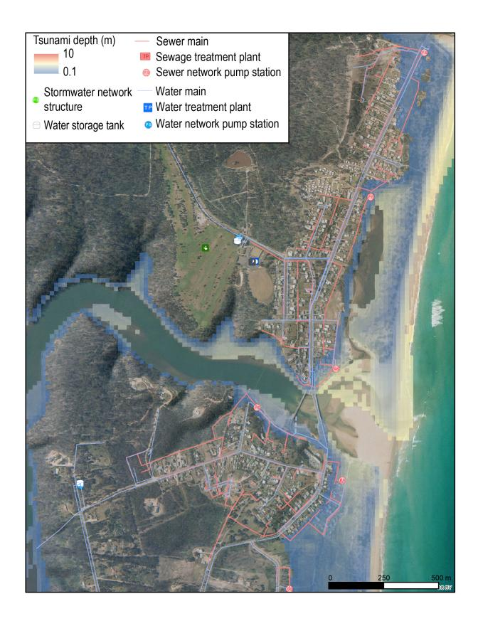
FIGURE 20: Map of infrastructure in the flooding zone at Scamander for PU3679. Data from ListData (2019).
