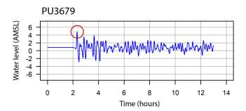
FIGURE 18: Simulated tsunami time series at Scamander. Maximum amplitude is circled in red.
