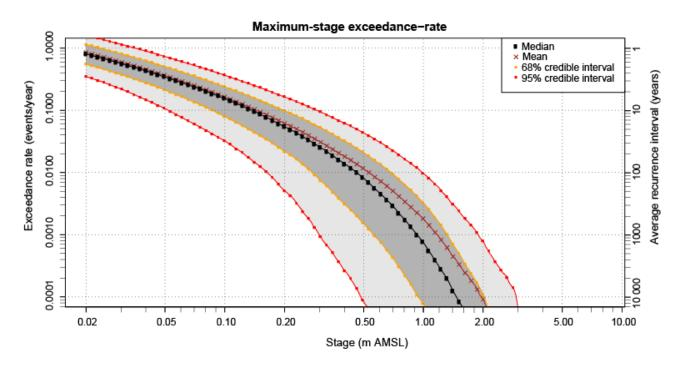
FIGURE 3: Plot of maximum-stage exceedance rates for PTHA Hazard Point 1552.1, which is located off the coast of Scamander where water depth is 103 m (at the model domain boundary in the central part of the study area). This is the same hazard point that is represented in Figure 4b.
