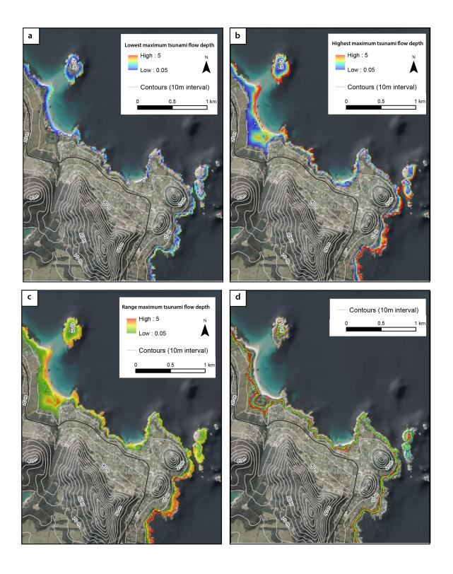
FIGURE 10: Variability between tsunami scenarios at Bicheno, showing the aggregated range of tsunami flow depths across all 20 scenarios. a) Lowest maximum tsunami flow depth. Note that the values for each cell may not be from the same scenario. b) Highest maximum tsunami flow depth. Note that the values for each cell may not be from the same scenario. c) Range of maximum tsunami flow depths. d) Inundation footprints of all 20 scenarios. See Appendix 3 for a more detailed image.
