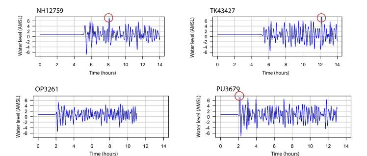
FIGURE 12: Simulated tsunami time series at Wineglass Bay for the four designated scenarios. Maximum amplitude is circled in red.
