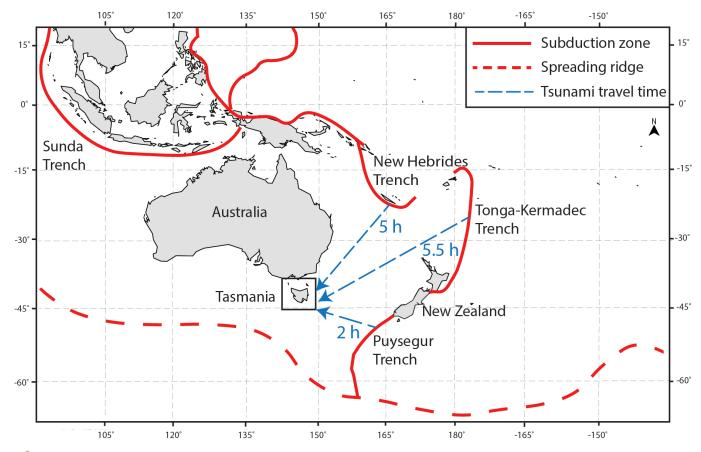
**FIGURE 2:** Location map of tsunami subduction source zones around Australia. Approximate tsunami travel times to Tasmania from the modelled source zones are shown in blue.
