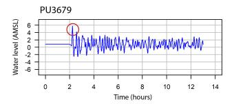
FIGURE 16: Simulated tsunami time series at Lagoons Beach. Maximum amplitude is circled in red.
