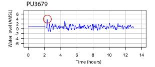
FIGURE 26: Simulated tsunami time series at Policemans Point, near Ansons Bay. Maximum amplitude is circled in red.
