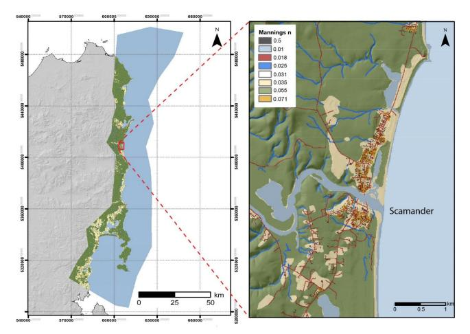
FIGURE 7: Manning's n zones as applied across the model domain, with a detailed example of the Scamander area.
