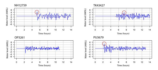
FIGURE 22: Simulated tsunami time series at larapuna (Bay of Fires). Maximum amplitude is circled in red.
