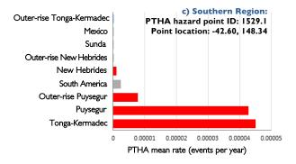
FIGURE 4: Regionspecific spatial hazard deaggregation for an ARI 10 000 year tsunami. a) North, b) Central, c) South. These plots describe
