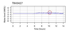
FIGURE 25: Simulated tsunami time series at St Helens township, highlighting the magnitude of wave attenuation within Georges Bay when compared with Figure 22. Maximum amplitude is circled in red.
