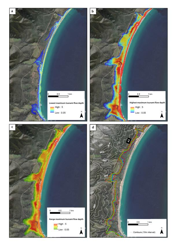
FIGURE 11: Variability between tsunami scenarios at Lagoons Beach, showing the aggregated range of tsunami flow depths across all 20 scenarios. a) Lowest maximum tsunami flow depth. Note that the values for each cell may not be from the same scenario. b) Highest maximum tsunami flow depth. Note that the values for each cell may not be from the same scenario. c) Range of maximum tsunami flow depths. d) Inundation footprints of all 20 scenarios. See Appendix 3 for a more detailed image.
