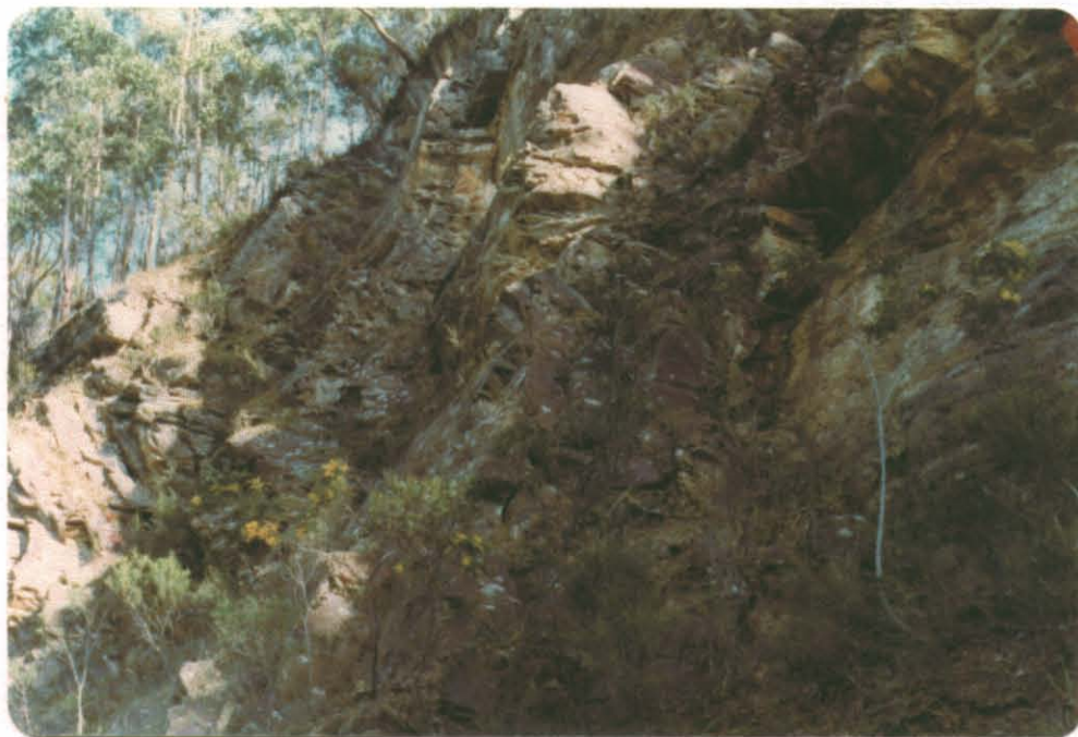
Plate 9. Wedges which have failed on a major joint dipping NE, and three bedding planes forming a large wedge failure unit.
