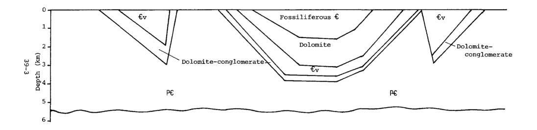
Figure 2. Interpretive cross-section of gravity data along line 480 000 m North between 300 000 and 360 000 m East. Density: Precambrian basement 2.67  $t/m^3$ ; dolomite-conglomerate succession 2.79  $t/m^3$ ; Volcano-sedimentary succession 2.70  $t/m^3$ ; upper dolomite succession 2.79  $t/m^3$ ; fossiliferous siltstone-mudstone succession 2.67  $t/m^3$
