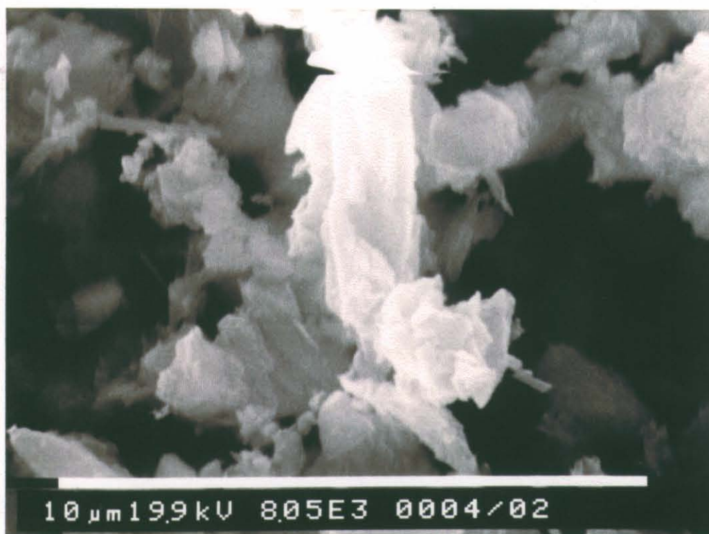
SEM photograph of an asbestos fibre on a Millipore membrane filter, Sample 107, drill 45R2, South Lens. Magnification: 8050x, scale bar = 10 µm.
