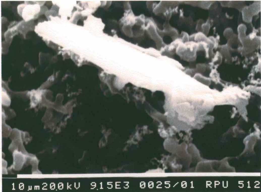
SEM photograph of asbestos fibres on a Millipore membrane filter, Sample 19, PH 1 shovel, Centre Deposit. Magnification: 9150x, scale bar = 10 µm.
