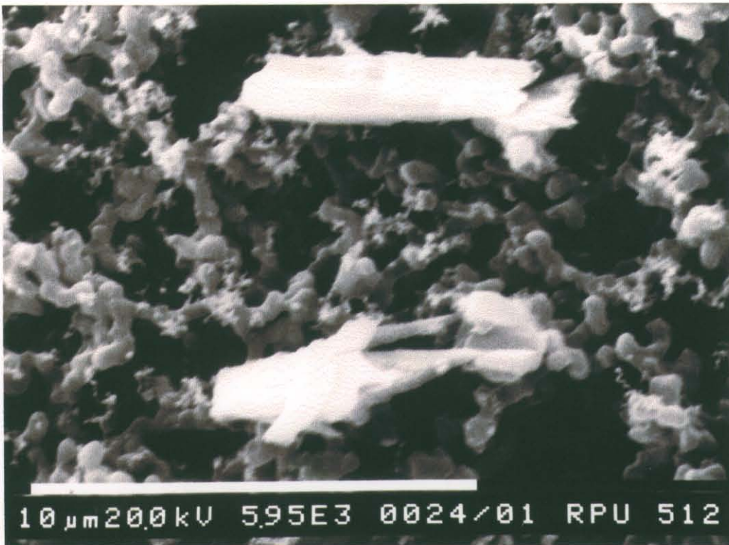
SEM photograph of an asbestos fibre on a Millipore membrane filter, Sample 19, PH 1 shovel, Centre Deposit. Magnification: 5950x, scale bar = 10 µm.
