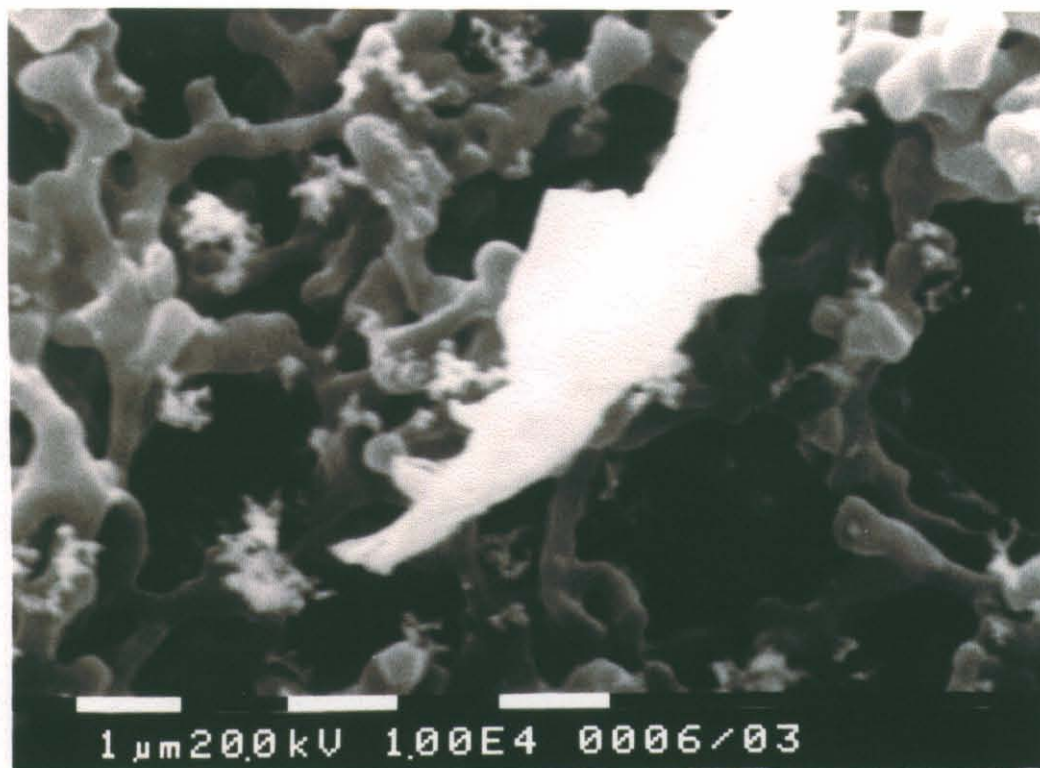
SEM photograph of asbestos fibres on a Millipore membrane filter, Sample 113, crusher cab. Magnification: 10 000x, scale bar = 1 µm.
