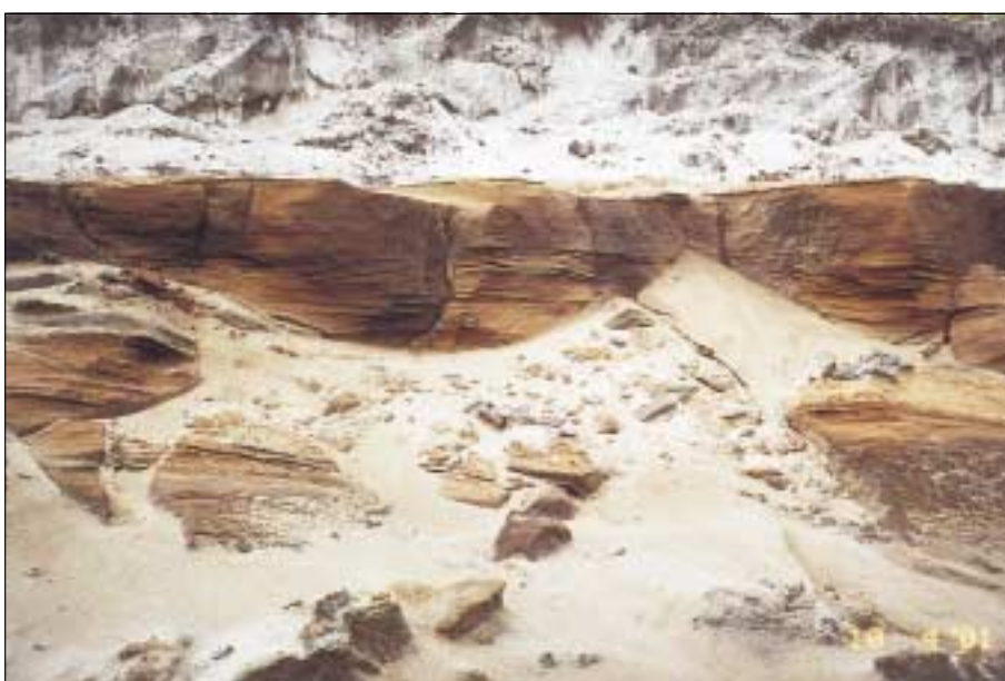
Plate 6. Potential acid sulphate soil layers in the channel excavation shown in Plate 5, northwest Tasmania
