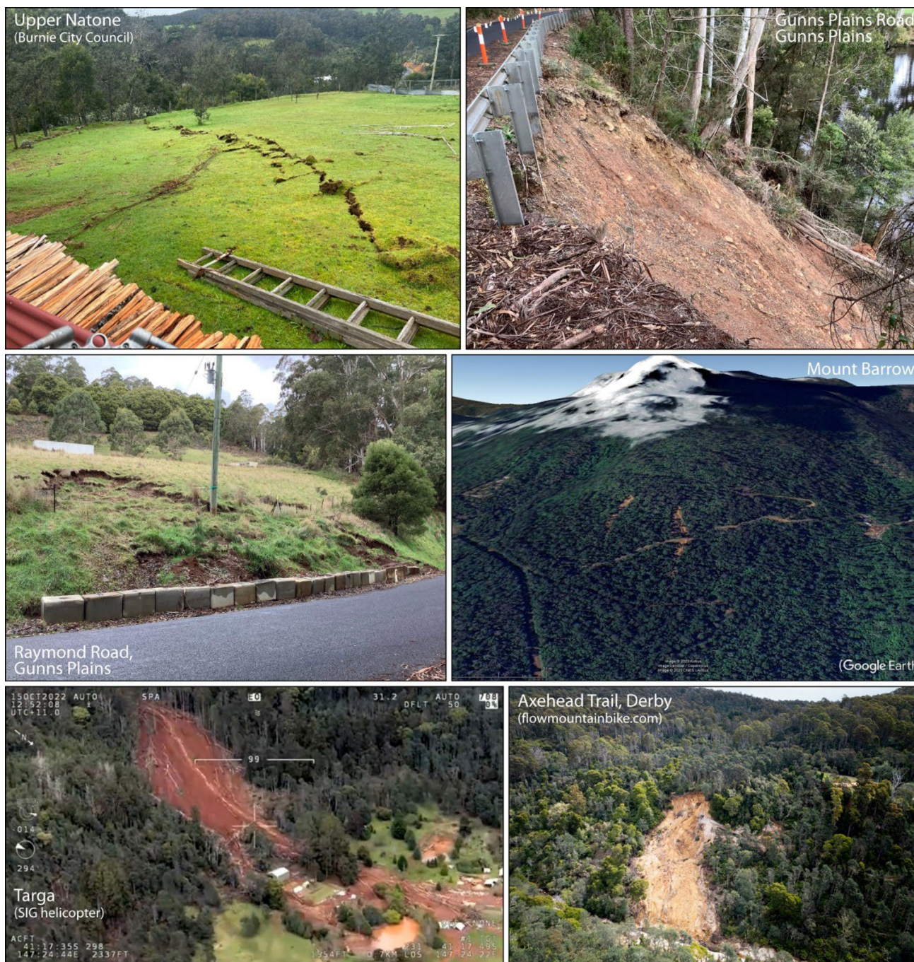
Figure 3. Various 2022 rainstorm-related landslides beyond the Great Western Tiers. These failures variously involved sliding, flow, and fall of debris (a mixture of soil, rock, and sometimes organic material) mantling slopes. Their velocities differ depending largely on landslide type, ranging from creeping to many kilometres per hour. Photos are from MRT field visits, unless otherwise attributed.
