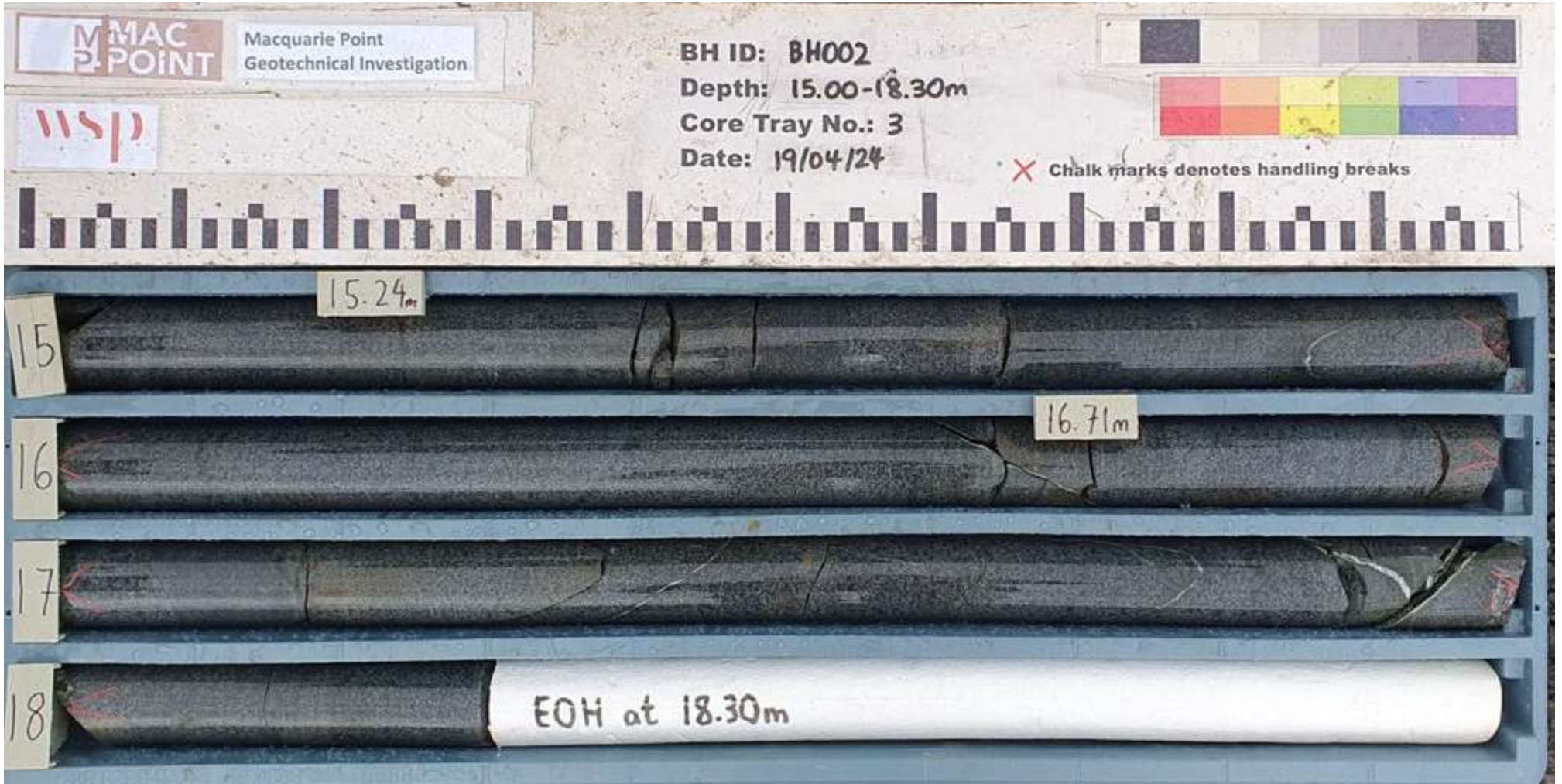
PointID : BH-002 Depth Range: 15.00 - 18.30 m
