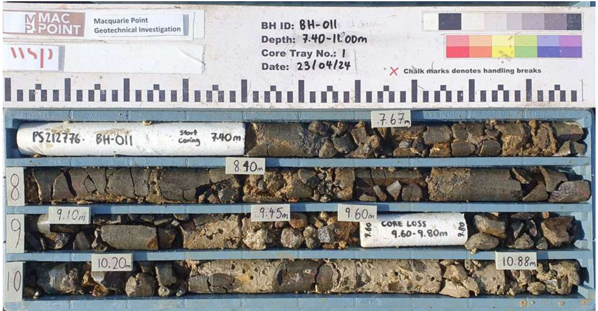
PointID : BH-011 Depth Range: 7.40 - 11.00 m
