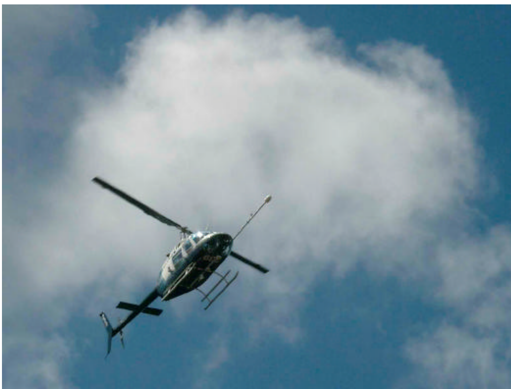
Figure 3a Helicopter with stinger instrument mount
