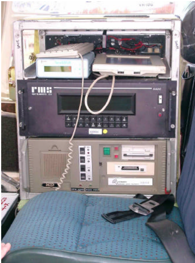
Figure 3c Helimag data acquisition unit
