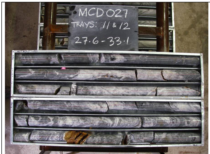
Intensely barite veined core from the main body of mineralization.
