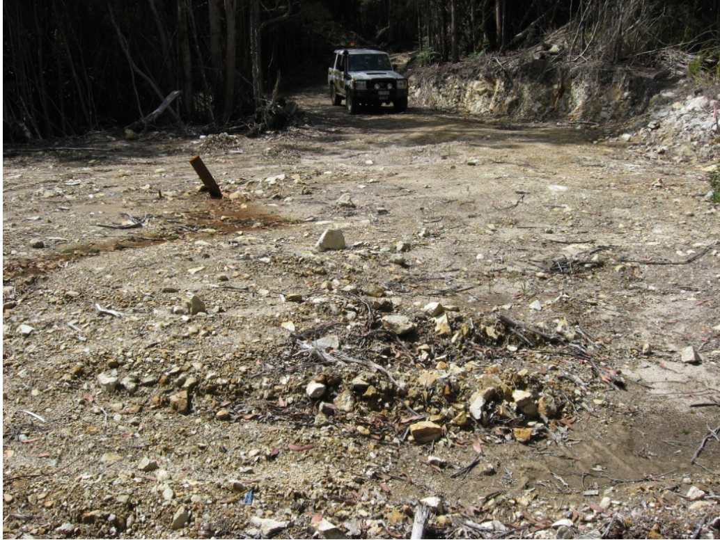
BHD-9 site – note lack of stockpiled material around pad. Collar is not leaking.
