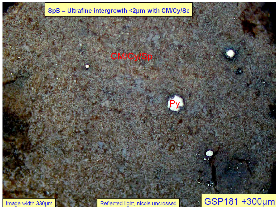
Figure 9B From G. McArthur: Major sphalerite type in Pits 170 & 264. CM = Carbonaceous Matter.
