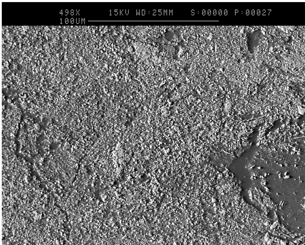
Figure 8. From S. McKnight: Detail fragment 2 – sphalerite in organic matrix.
