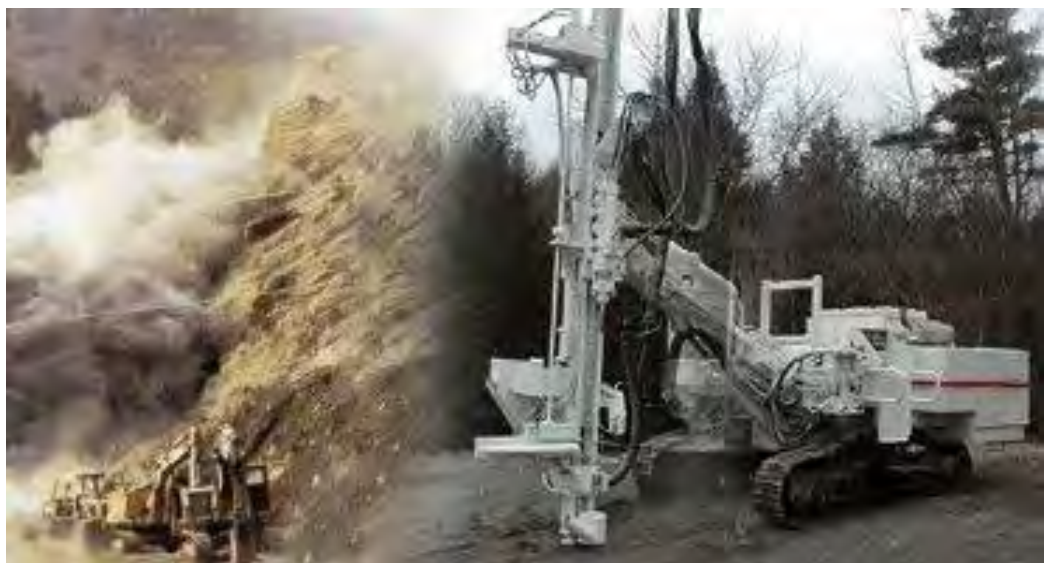
Figure 3-1 Drill and Blast Mining Equipment
