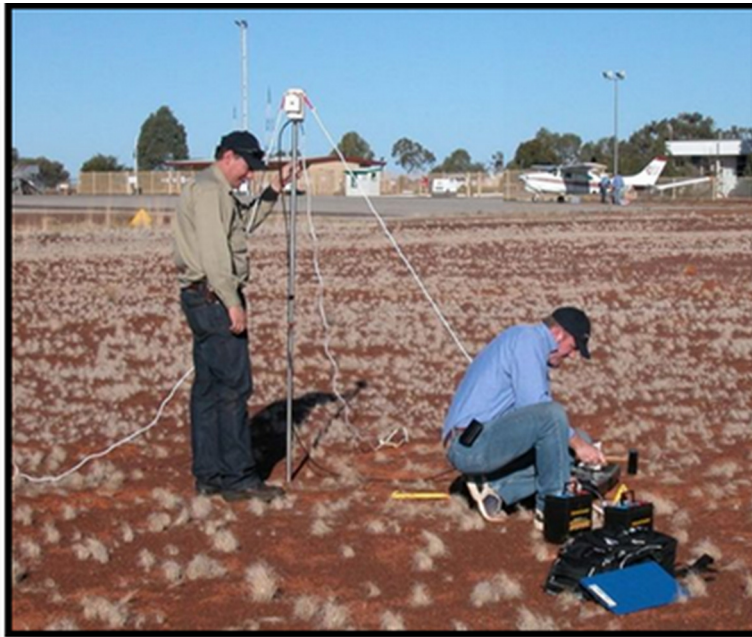
Figure 11 Setting up base station magnetometer
