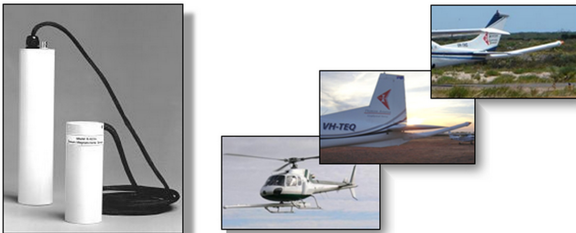
Figure 5 G822A Magnetometer and Typical Stinger Mounts
