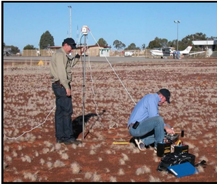
Figure 11 Setting up base station magnetometer
