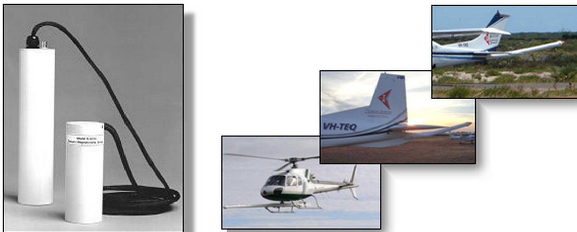
Figure 5 G822A Magnetometer and Typical Stinger Mounts
