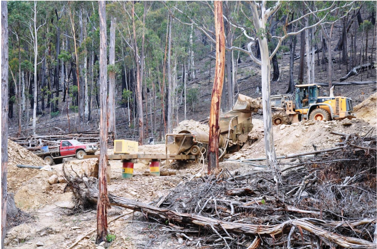
Figure 4.1: Alluvial treatment plant in Grants Gully with loader feeding screen leading into sluice.
