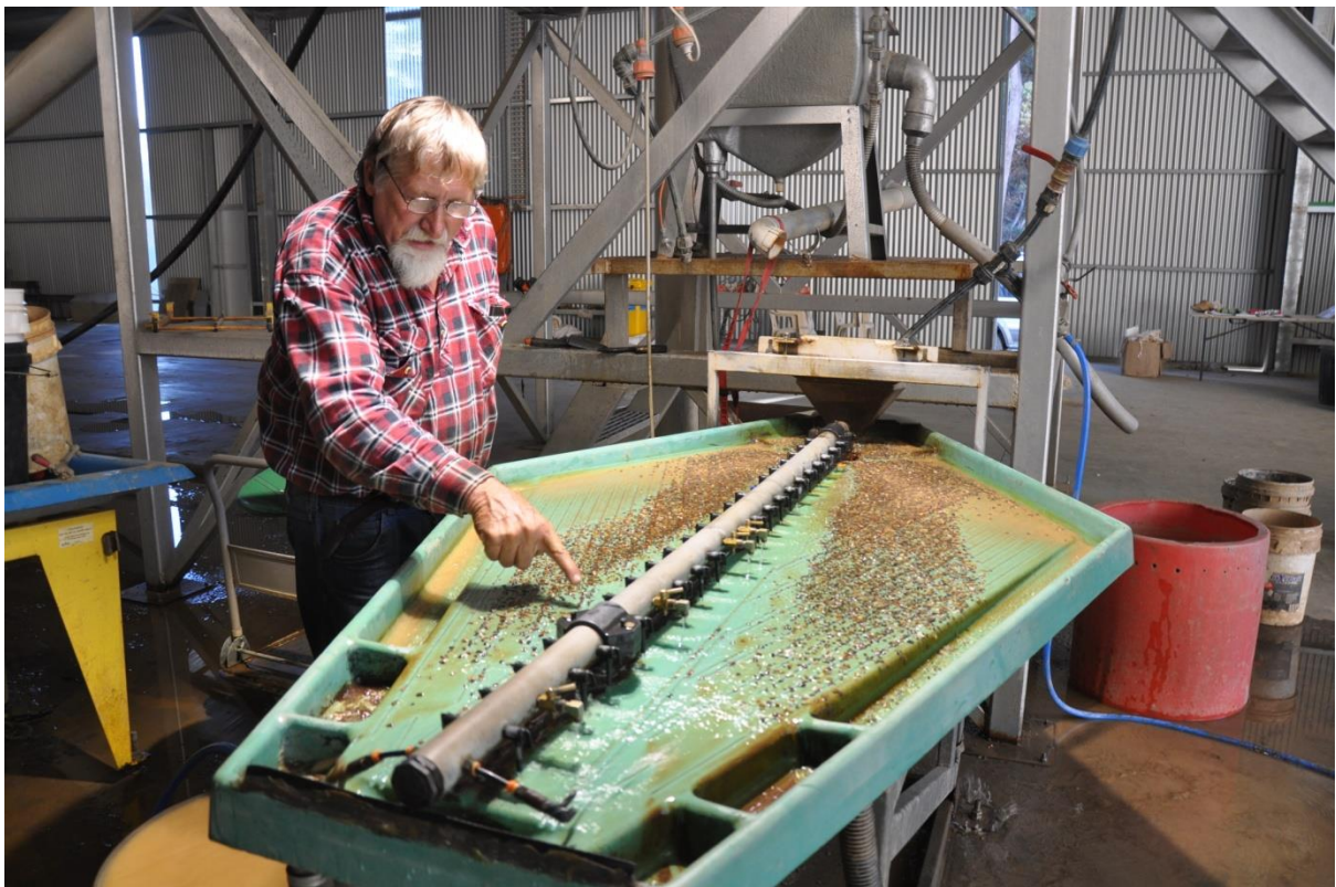
Figure 4.2; Steve Parker operating gemini table at sailors Gully mine/mill site.
