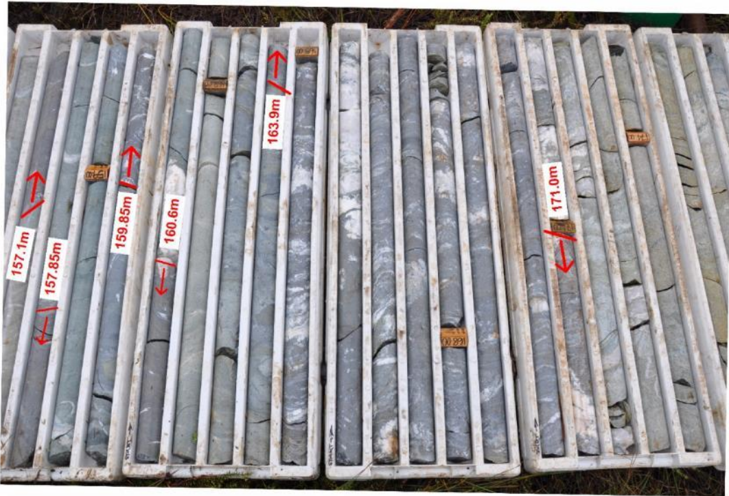
Figure 2.3: WD025 drillcore showing high grade base metal massive sulphides from 157.1m to 157.85m, 159.85m to 160.6m and 163.9m to 171.0m.
