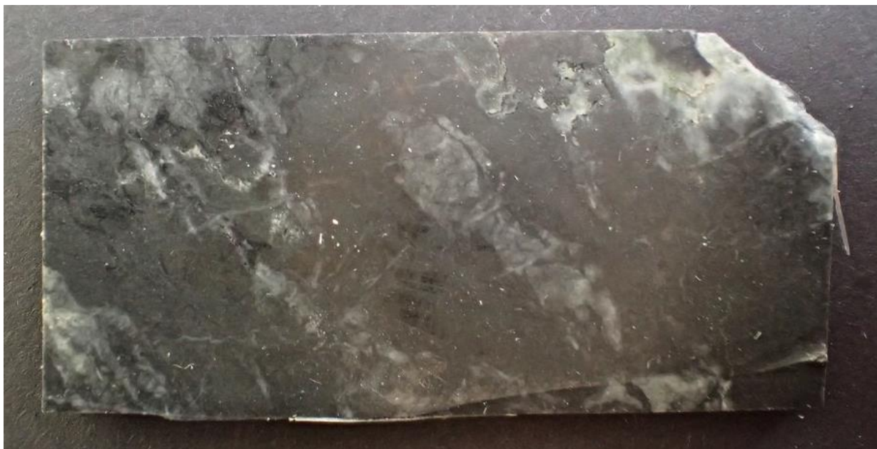
Fig. 25. Sample G409087, Mottled pale grey-white hornfels, Plain light, FOV (field of view) ~90mm.
