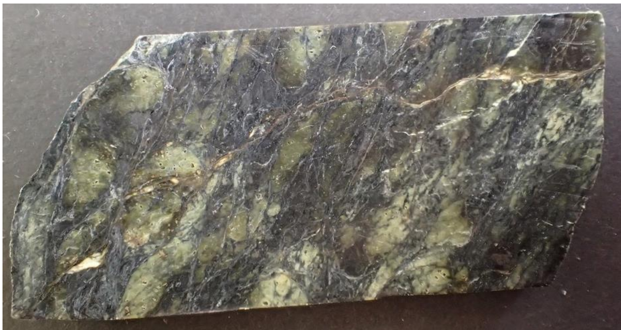
Fig. 16. Sample G409085, Clastic-textured serpentinite, with veins. Plain light, FOV (field of view) ~90mm.
