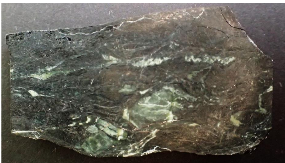
Fig. 1 Sample G409083, Clastic-textured serpentinite, sheared and veined. Plain light, FOV (field of view) ~80mm.
