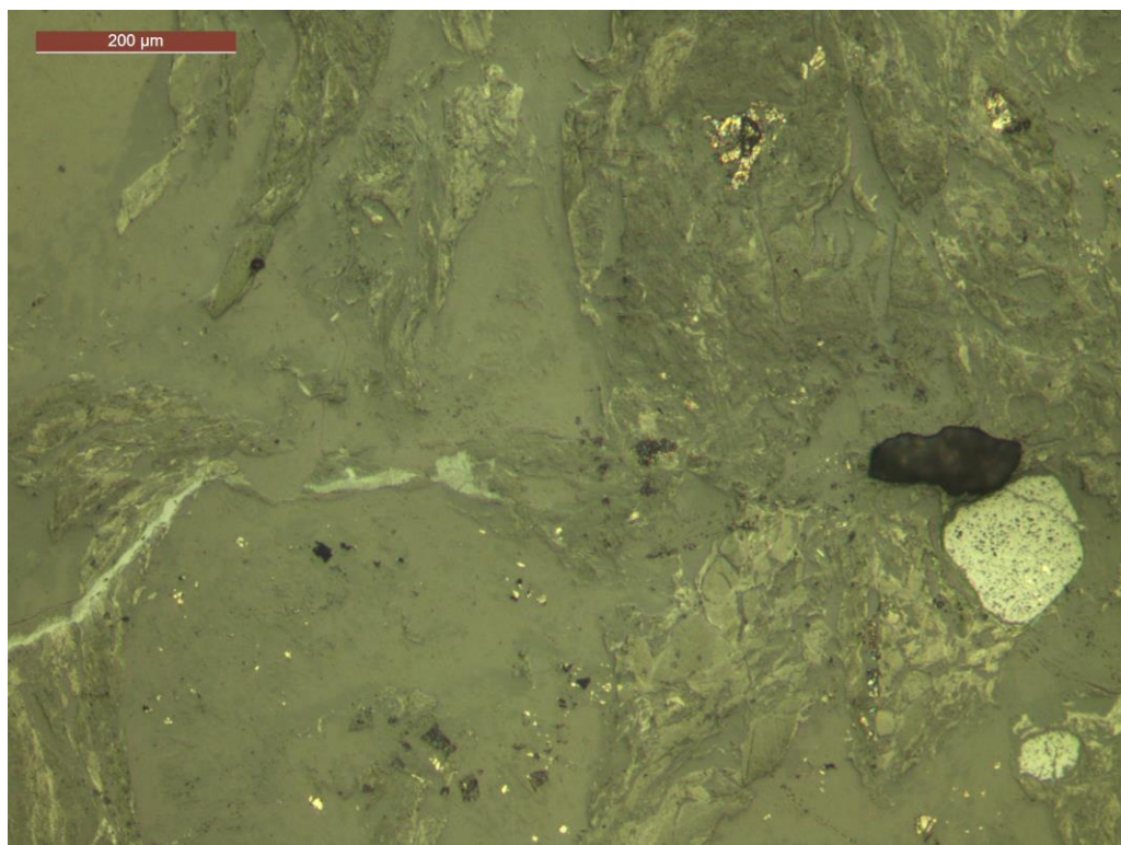
Fig. 6. Sample G409083, Polarised reflected light, plain polars, showing bright grey magnetite aggregates after chromite (lower RHS), a blue-grey limonite vein (centre left), diffuse medium grey patches of very fine grained magnetite, and some small patches of yellowish haalpaite(? , upper right) in a dark grey serpentine matrix.
