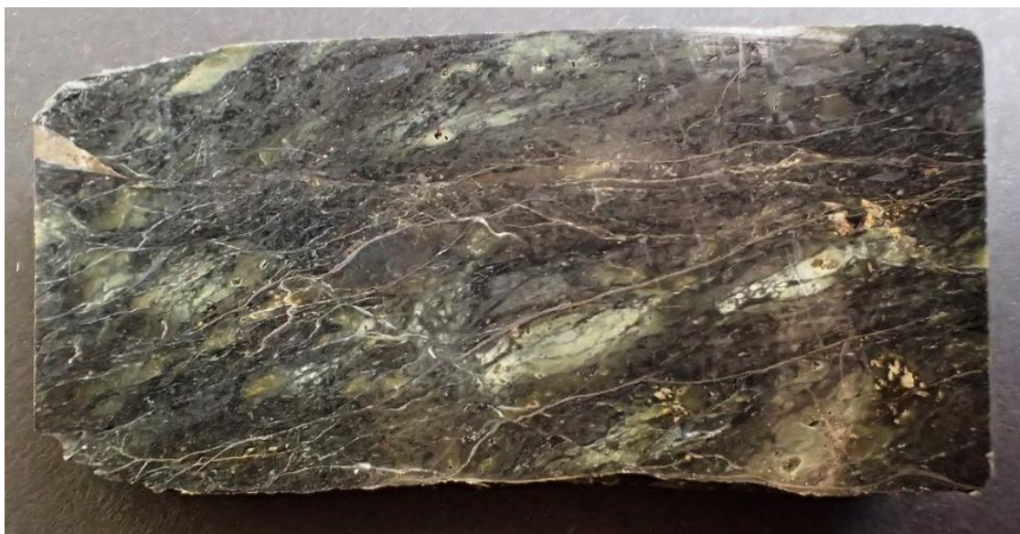
Fig. 22. Sample G409086, Clastic-textured serpentinite, Plain light, FOV (field of view) ~90mm.
