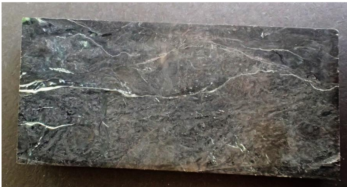
Fig. 9. Sample G409084, Breccia-textured serpentinite, Plain light, FOV (field of view) ~90mm.
