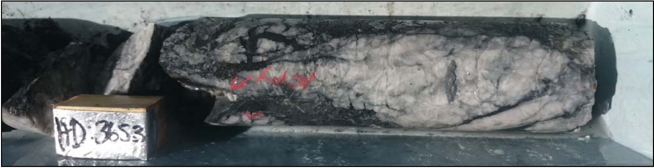
Photo 2. MDD006 - Quartz Vein Breccia and Minor Sulphides at 365.3m.
