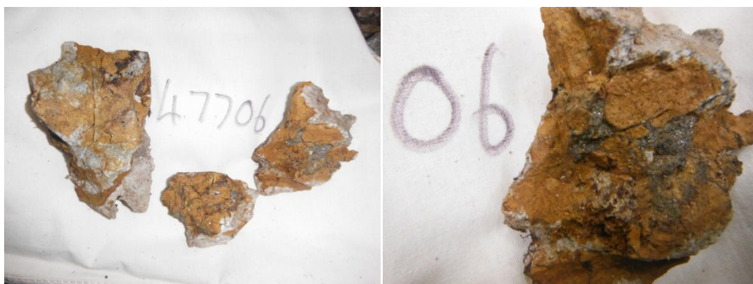
Photo 1: Sample 47706; FeO haloes on irregular stringer pyrite veining.
