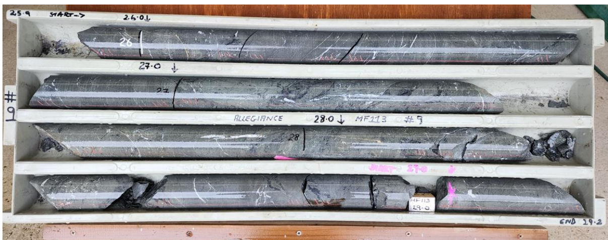
Figure 11. Typical quartz-carbonate veined greywacke intersected at Scout Camp.
