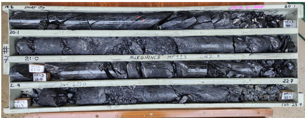
Figure 10. Typical pyritic-pyrrhotitic-graphitic black shales intersected at Scout Camp.
