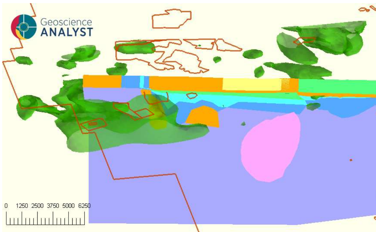
Figure 31: Lemont 3D MT model isosurface (green; 500 Ohm.m) clipped N and S and intersected with the 2.5D gravity model, Section 4. View from the north, see Figure 29 for section location. Unit colours as per 1:250000 geology map.
