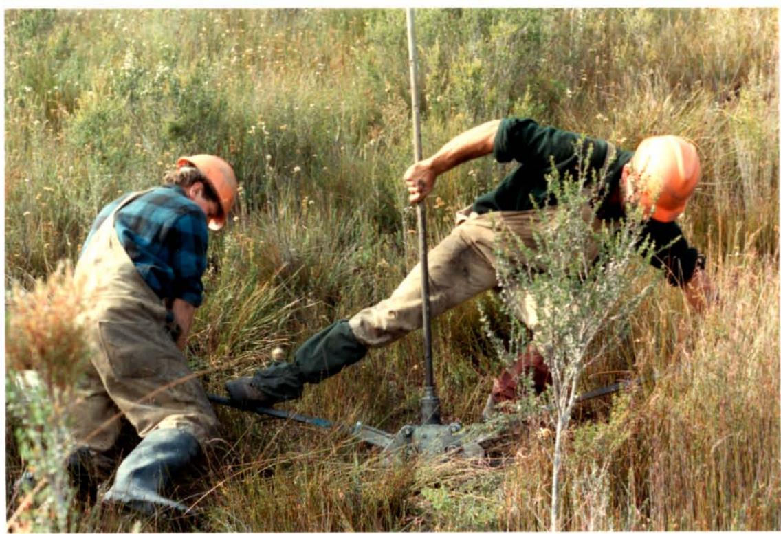
4b Jacking rods and sample tube out of hole.
