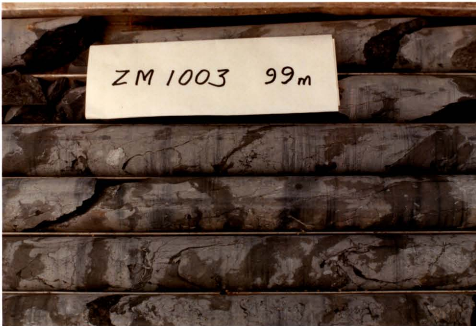
3a "Patchy Limestone" - darker patches calcareous dolomite, lighter patches weakly dolomitic bioclastic wackestone.
